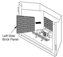
Figure 43 - Installing Side Brick Panels
