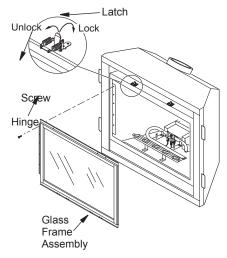
Figure 41 - Removing/Replacing Glass
