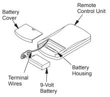
Figure 39 - Installing Alkaline Battery in Hand-Held Remote Control Unit
