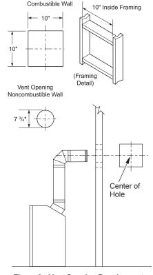
Figure 9 - Vent Opening Requirements
