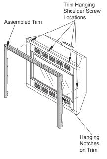
Figure 51 - Attaching Trim to Firebox
