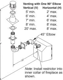
Figure 22 - Vertical Venting Configuration Using One 90° Elbow (Vertical Round High Wind Termination Shown)
