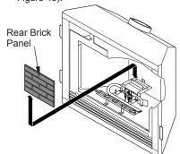
Figure 42 - Installing Rear Brick Panel
