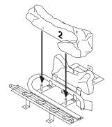
Figure 45 - Installing Log No. 2
