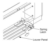
Figure 40 - Removing Louver Panel
