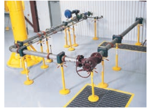
In addition to testing chokes over a wide range of pressures, Cameron measures flow rates and noise in a flow loop per ISA specifications.
