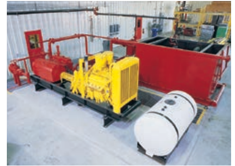
Cameron has an extensive erosion test facility with specially designed equipment yielding high differential pressure capabilities, as well as variable abrasive content flow.
