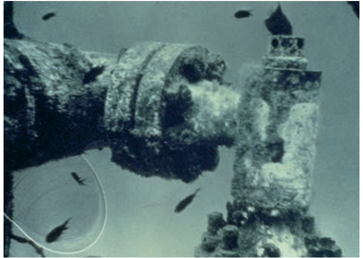
The first Cameron subsea choke supplied in 1975, installed in the Gulf of Mexico.
