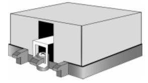
2. After tightening screws secure metal clip to plastic retention bracket center tab. Repeat for the other side of heatsink.
