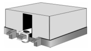
1. After placing CPU back-plate and adhesive interface material under motherboard, place heatsink retention frame on top of motherboard. Align heatsink retention frame screw hole with backplate assembly standoffs. Place heatsink inside plastic retention bracket. Place metal clip over retention frame tab. Repeat for other side.
