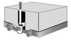
2. Insert screw through metal clip. BE SURE METAL CLIP IS LOCKED ONTO RETENTION FRAME TAB.
