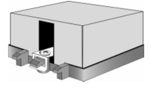
Tighten screw through metal clip.
