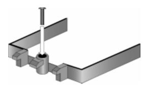
1. After placing backplate and interface material under motherboard place heatsink retention frame on top of motherboard. Align plastic retention bracket screw holes with CPU backplate standoffs.
