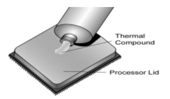
There are two types of thermal interface materials designed for use with the AMD<sup>®</sup> Athlon64<sup>™</sup> / Opteron<sup>™</sup> 1xx 939-pin series processors.
