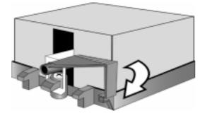
3. After securing metal clip to plastic retention bracket center tab, push down on plastic clip to lock plastic clip to side tab.
