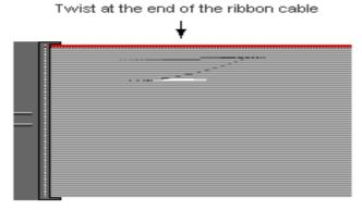
Attach first floppy drive (drive **A**:) to the end of the cable with the twist in it. Drive **B**: is usually connected to the next possible connector on the cable (the second or third connector after you install Drive **A**:).
