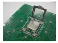
7. Close the socket. Rotate the load plate onto the package lid.
