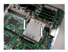
**NOT**E: The back plate is already mounted on the backside of mainboard. You don't need to pay additional attention on mounting the back plate.
