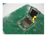
Locate the Pin 1 indicator of the package. Align the package with the socket and carefully insert the package into the socket with vertical motion only. Vertically check if the CPU is seated well in the socket housing. If not, take out the CPU, with vertical motion only, and repeat the above steps.
