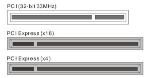
Simply find the appropriate slot for your add-in card and insert the card firmly. Do not force any add-in cards into any slots if they do not seat in place. It is better to try another slot or return the faulty card rather than damaging both the motherboard and the add-in card.
