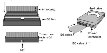
Simply plug in the BLUE END of the IDE cable into the motherboard IDE connector, and the other end(s) into the drive(s). Each standard IDE cable has three connectors, two of which are closer together. The BLUE connector that is furthest away from the other two is the end that connects to the motherboard. The other two connectors are used to connect to drives.
