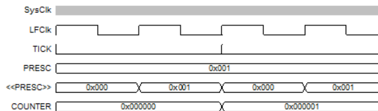
Figure 33: Timing diagram - COUNTER_PRESCALER_1
