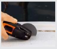
The round HSS saw blades are excellent for sawing work on fibreglass and carbon fiberglass reinforced plastic hulls. Make perfectly clean cuts (0.5 mm wide) without any cracking or damage to the laminate.
