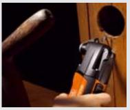
The MINICUT saw blades are exactly the right size for working in tight spaces, difficult-toreach spots or for sawing small recesses (above  $\frac{3}{3}$ ").
