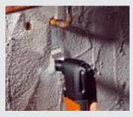
Ideal for dismantling installations that are no longer required. Using the universal E-CUT saw blades the pipes are clipped off for subsequent grouting flush to the wall.
