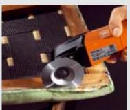
The flush cut HSS saw bladesaves you effort and the upholstery, as staples can be easily removed and do not have to be pulled out with pliers.
