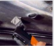
Even stubborn undercoatings can be removed easily with the rigid scraper blade in the fastest possible time.
