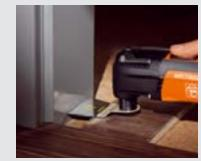
The high precision and cutting speed of the E-CUT saw blades are impressive when altering door jambs for higher floor coverings or making recesses in parquet and laminate.
