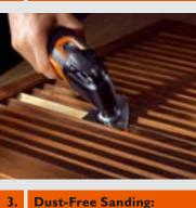
The flat sanding pad also gives access to tight spaces, e.g. the slats of shutters.
