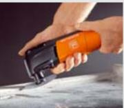
Renovate very old windows perfectly and work effortlessly into corners with the HSS segment saw blade.
