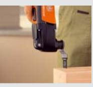
Saw into wood 2  $3\%^{\prime\prime}$  deep with the new universal E-CUT saw blades.
