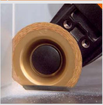
The segment saw blade is used for removing defective tile joints in corners and on edges accurately and without overcutting. It is available in carbide or diamond quality; the latter will impress you with its noticeably higher service life and is also suitable for epoxy resins.
