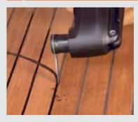
Remove deck sealing materials quickly and thoroughly with the cutting blades. The time saving is 80% and more when renovating teak decks.
