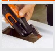
Recesses can be filed precisely to shape with the MINICUT and File Set.
