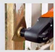
With the carbide rasp, remove stubborn signs of weathering thoroughly and quickly thanks to the high sanding capacity.
