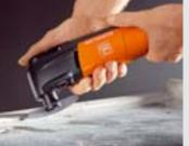
Brittle puttied edges can be removed without any problem and without any danger of glass breakage.
