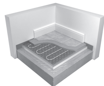
Lay the pipe
