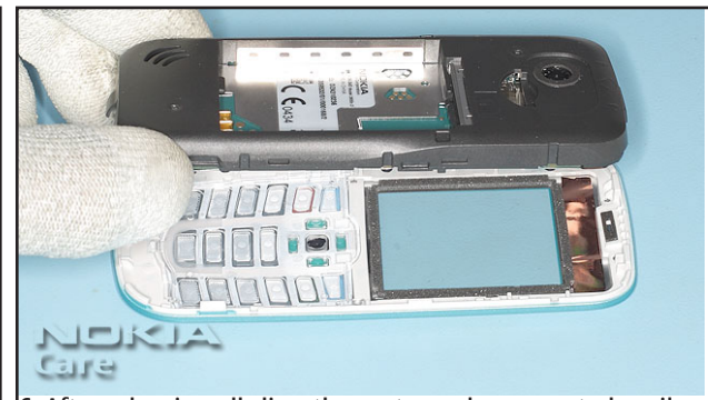
6. After releasing all clips, the parts can be separated easily.
