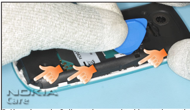
5. Also release the 3 clips at the opposite side, starting at the top. Do not bend the A-COVER while releasing the clips.
