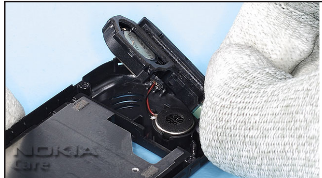
18. Lift out the IHF ANTENNA MODULE.
