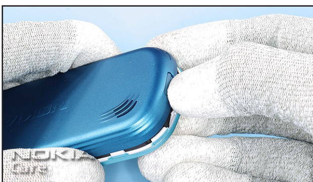
3. Unlock and remove the B-COVER.
