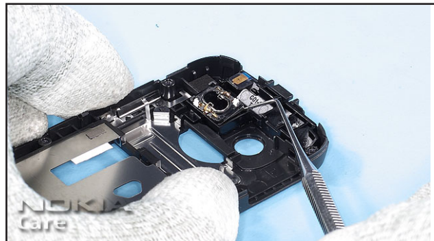
20. Gently lift out the EARPIECE. Also remove the adhesive residues from the opponent part.
