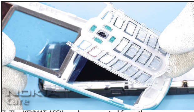
7. The KEYMAT ASSY can be separated from the cover.
