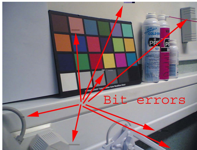
Figure 105 Bit errors caused by JPEG compression
