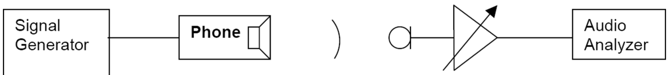
Figure 21 Test arrangement for of earpiece
