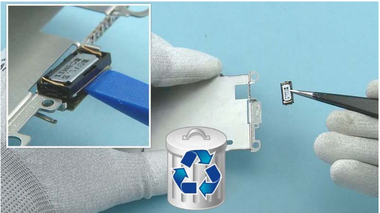
24) Release the EARPIECE with the SS-93 and remove it with tweezers. Do not use the EARPIECE again. Discard it.
