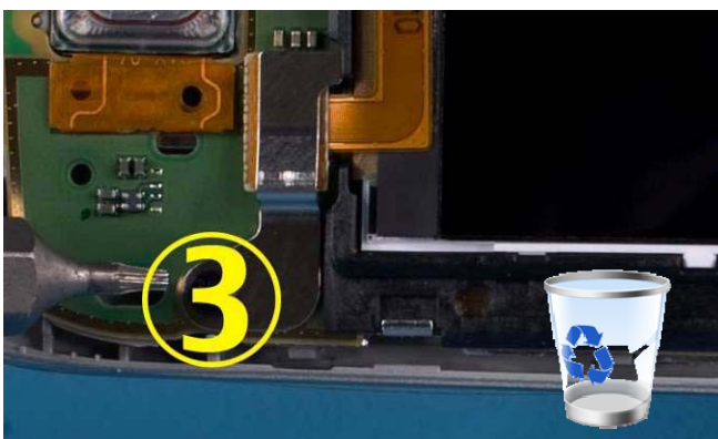
11) Use TORX 4 screwdriver to unscrew AUSTRALIA CONNECTOR BRACKET screw. Do not use screw again.
