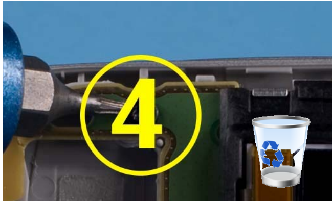
13) Remove the remaining screw on the PWB with TORX 4 screwdriver.
