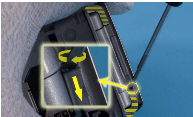
3) Insert small flat head screwdriver and turn clockwise to release SCREW CAPS.
