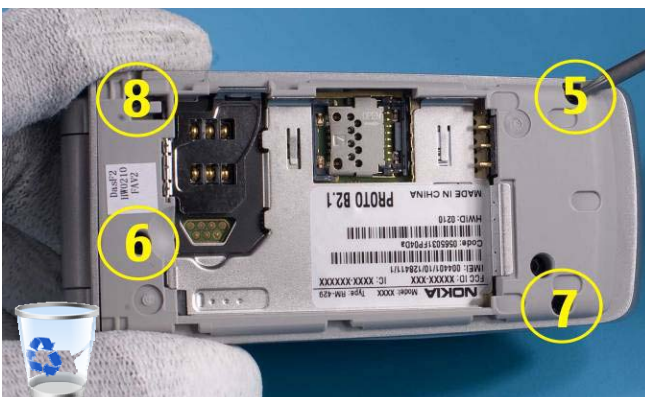
29) Remove 4 Screws with TORX 6 Screwdriver in the order as shown.
