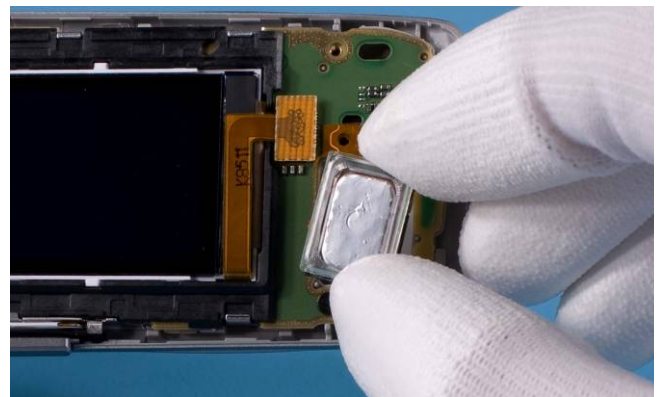
10) Lift up and remove IHF SPEAKER.
