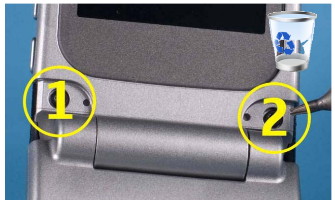
4) Use TORX 4 screwdriver to remove 2 screws. Do not use them again.
