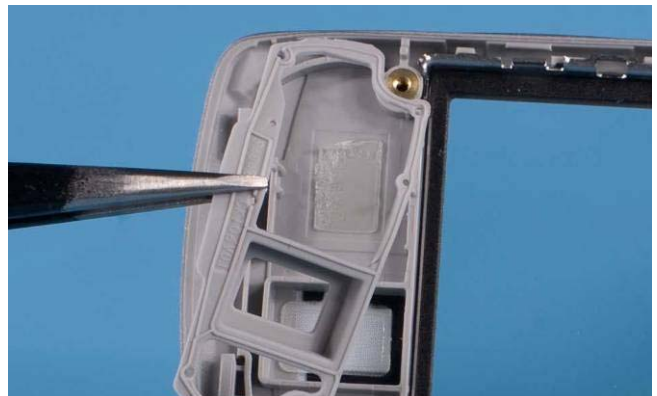
28) Use tweezers to remove IHF SPEAKER GASKET.
