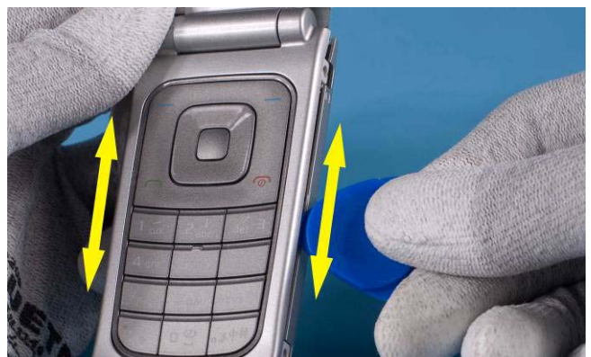
30) Insert SRT-6 Tool to slide along edges to release Tabs on both sides.
