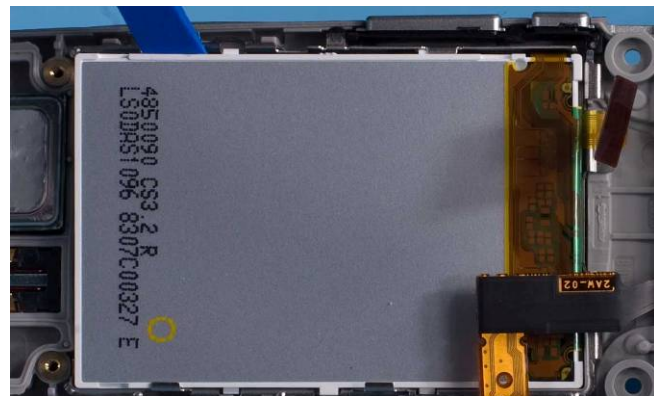
24) Use SS-93 tool to release tabs from LCD.
