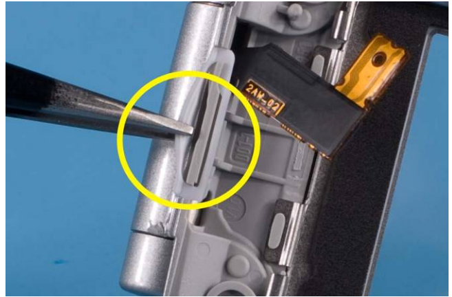
38) Remove DAMPER with Tweezers.
