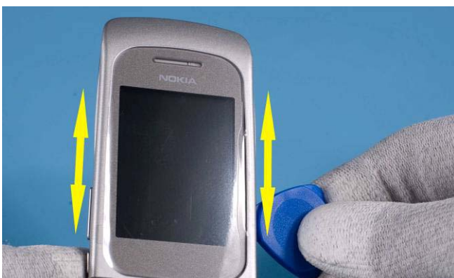
5) Insert SRT-6 tool and slide along edges to release tabs on both sides.
