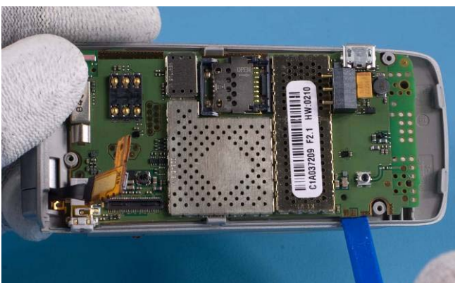
35) Use SS-93 Tool to release Tabs from D-COVER.
