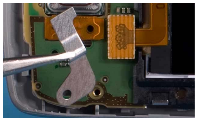
12) Use tweezers to remove AUSTRALIA CONNECTOR BRACKET.
