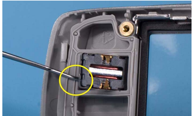
26) Use dental pick to release EARPIECE.
