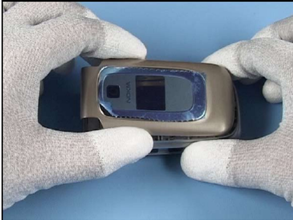
7. Shift the A-Cover to the hinge direction and lift it up.
