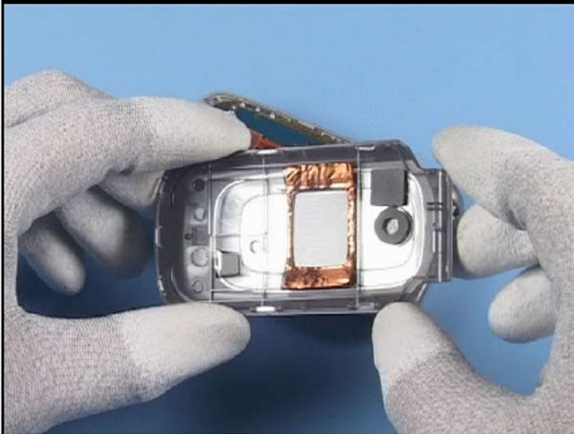
37. Fit a new SECONDARY GASKET to the B-COVER ASSEMBLY if not already done.
