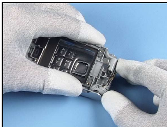
28. Now, the A-COVER UPPER ASSEMBLY can be removed easily. Mind the flex foil. Do not remove the tool, that locks the hinge yet.
