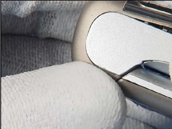
19. Click the snaps into their places, beginning from the upper side of the ANTENNA COVER.
