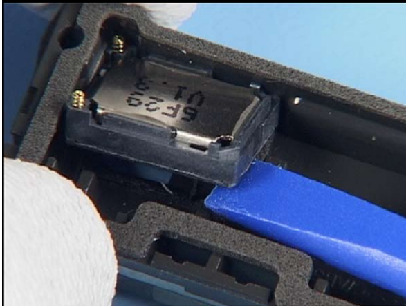
19. Lever out the IHF SPEAKER with the SS-93 first.
