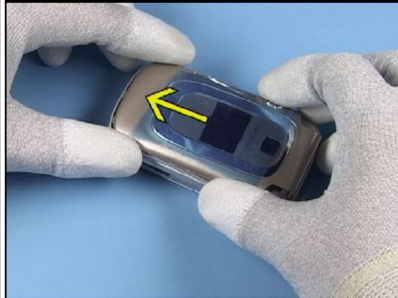
38. Place the B-COVER at the shown side first and shift it into the correct position.
