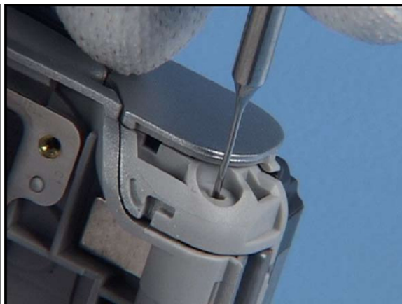
26. Bend down the hinge module with the SS-6 first. Note that the SS-6 is very delicate and can be break easily.
