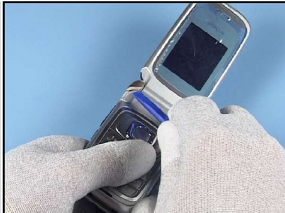
4. Open the assembly, release both upper clips of the ANTENNA COVER.
