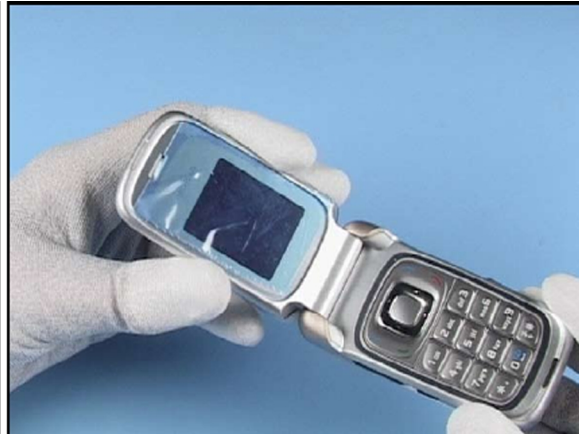
2. Cover the windows with a protective film.
