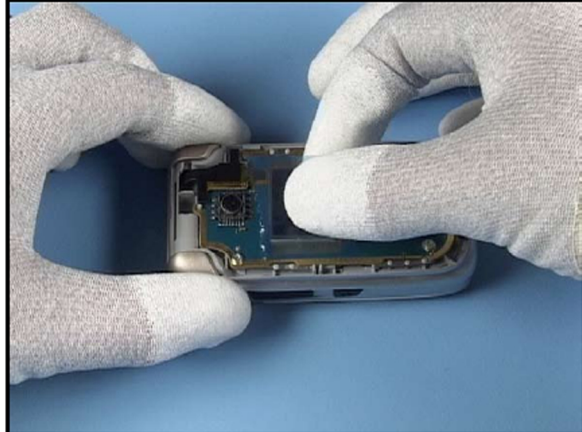
8. Cover the LCD PM with a protective film.
