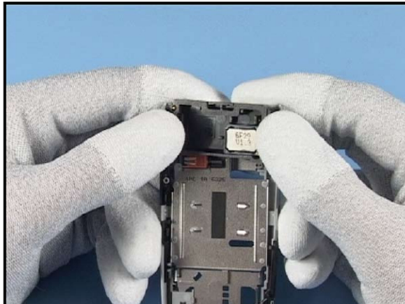
16. Carefully bend the C-COVER as shown to release the clips holding the ANTENNA COVER.
