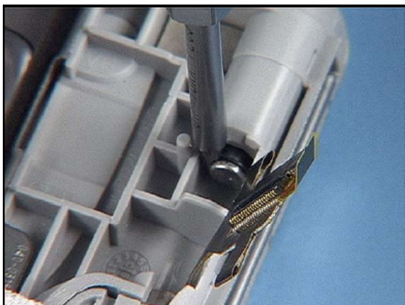
27. Now lock the HINGE with a torx bit size 6 or similar.
