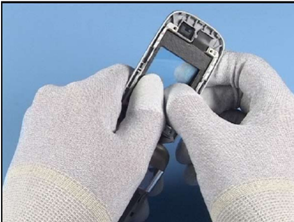
23. Push out the glued in LCD WINDOW.
