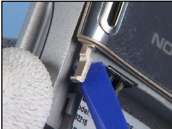
24. Unlock the clips of the ANTENNA CAP.
