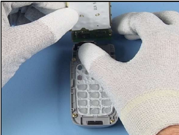
11. Bring the ENGINE MODULE into position near the hinge.
