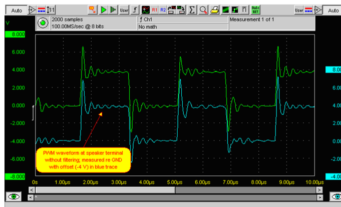
Figure 45 Differential output waveform of the Ext_in_IHF_out out loop measurement when speaker is connected.
