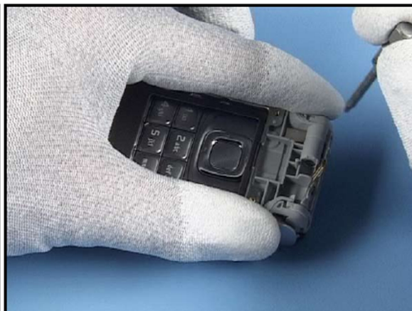
4. Now expand the HINGE MODULE by removing the tool.
