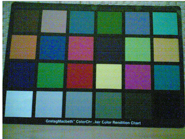
Figure 152 Noisy image taken in +70 degrees Celsius
