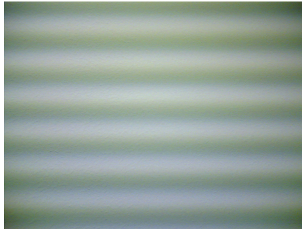
Figure 154 Flicker in an image; object illuminated by strong fluorescent light
