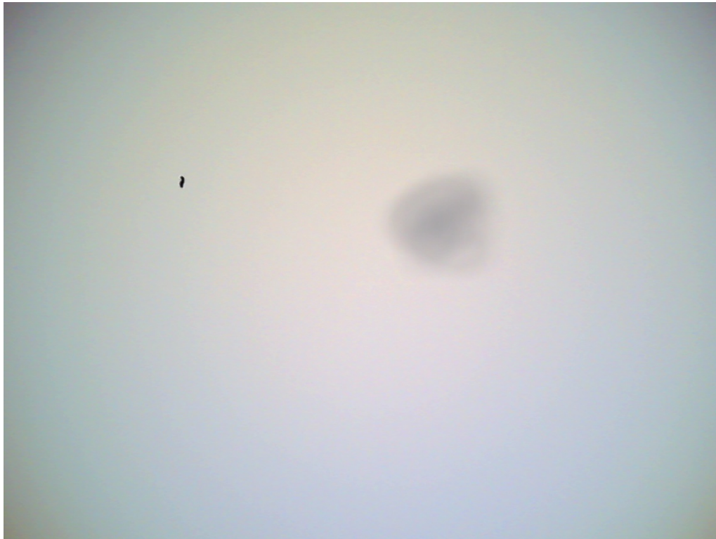
Figure 158 Effects of dust on optical path
