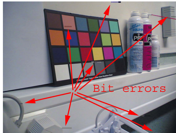
Figure 159 Bit errors caused by JPEG compression
