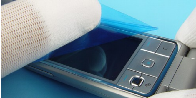
1.) Protect the WINDOW with a film to avoid dust and scratches.
