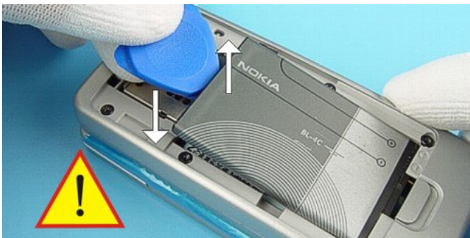
3.) Always remove the BATTERY before continuing disassembly.
