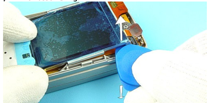
14.) Lever up the right corner of the LCD with SRT-6.
