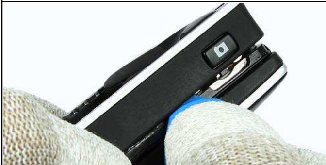
5.) Release the clips of the D-Cover.
