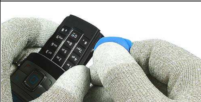
11.) Lever out the glued Keymat Assy.
