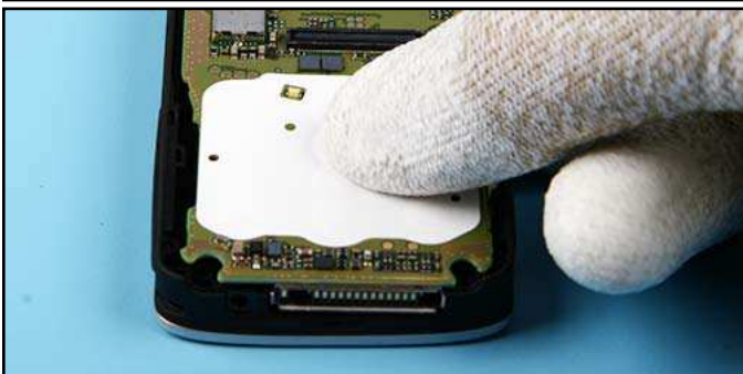
7. Finally, fix the MAIN DOMESHEET all-over.
