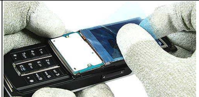
10.) Protect the LCD with a plastic film.
