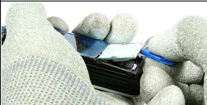
11.) Shift together the unit. Lift up the glued UI PWB Assy carefully with the SRT-6.
