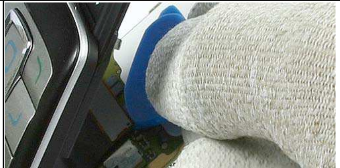
10.) Open the flex connector carefully.
