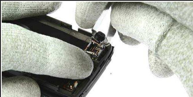
19.) Release the VGA Camera with the SS-51. Hold the Main Flex near the Camera Socket while removing the
