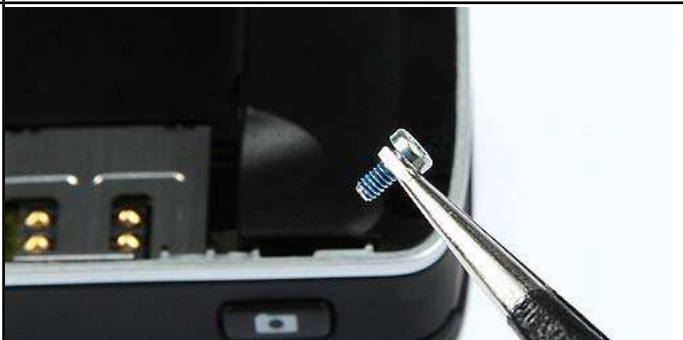
4.) Once removed, the screws can't be used again. Always use new screws for assembly.
