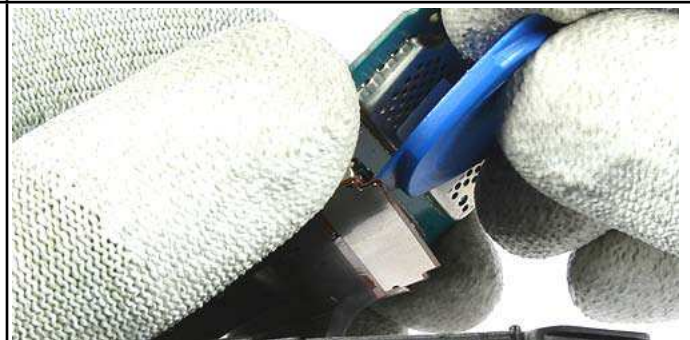
14.) Now release the other side of the flex connector.
