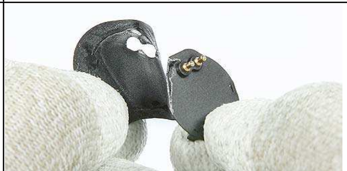
16.) Peel up the IHF Label completely. Always use a new one when reassembly. Ensure that no residues remain.
