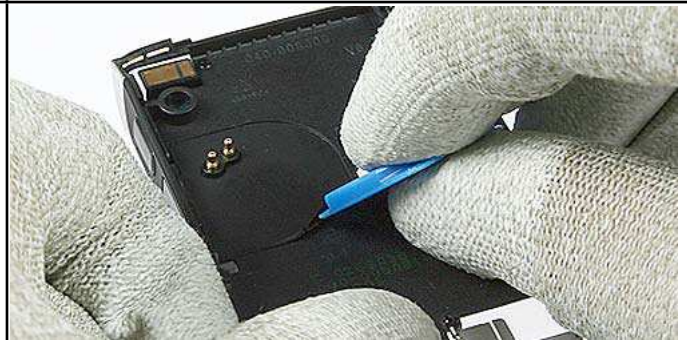
14.) Release the IHF Label with the SRT-6.
