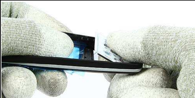
9.) Protect the inner side window with a plastic film. Remove the Keymat as shown.
