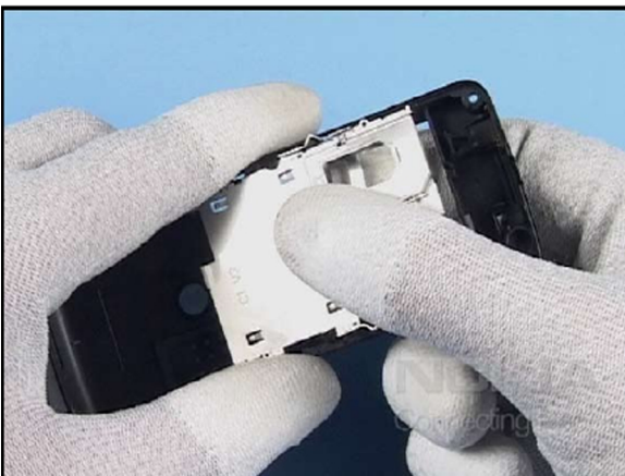
35. Release the LABEL COVER ASSEMBLY, beginning from the bottom side.
