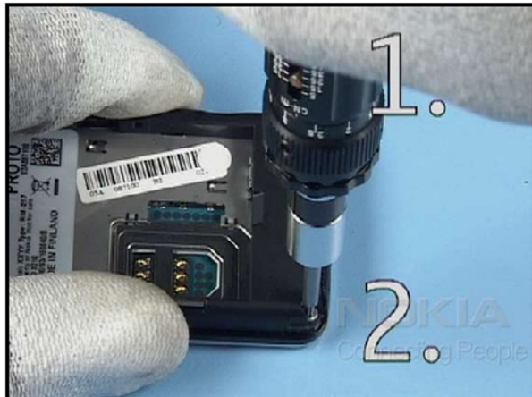
16. Tighten both screws of the C-COVER in the order shown, too.
