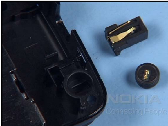
24. Remove the MICROPHONE and the DC JACK.
