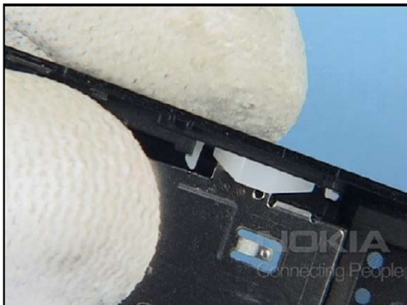
7. Insert the LED- and the SIDE- WINDOW. Note that they can't be interchanged.
