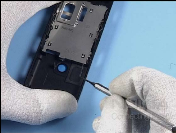
31. Release the shown metal snaps of the LABEL COVER ASSY with the dental pick.
