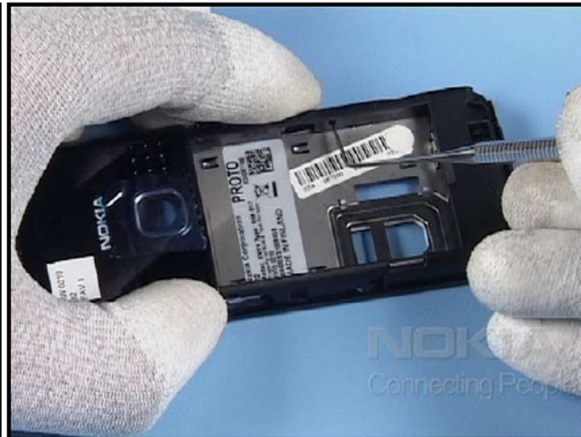
34. Use the dental tool to push out the last clips.
