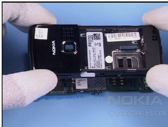
14. Turn the assembly, lift up the B-COVER.
