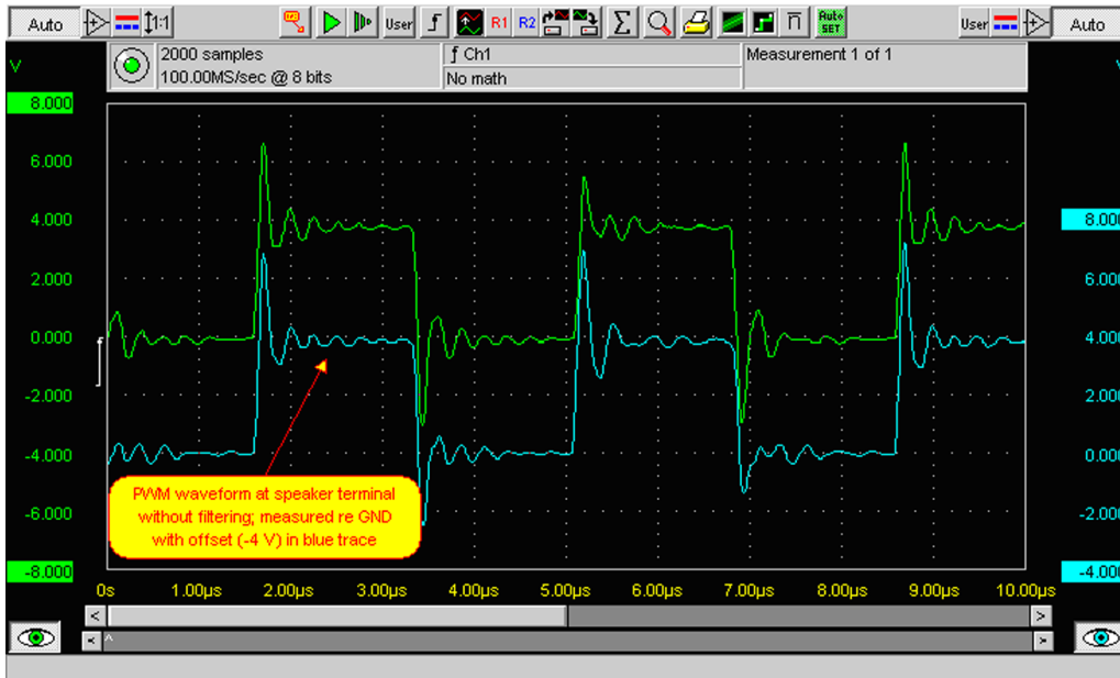
Figure 38 Differential output waveform of the Ext_in_IHF_out out loop measurement when speaker is connected.
