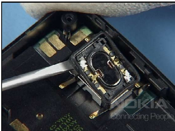
25. Carefully lever out the EARPIECE ASSEMBLY.
