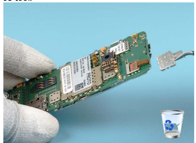
18b) Remove the FLEX SHIELDING with the tweezers. Do not use this part again.
