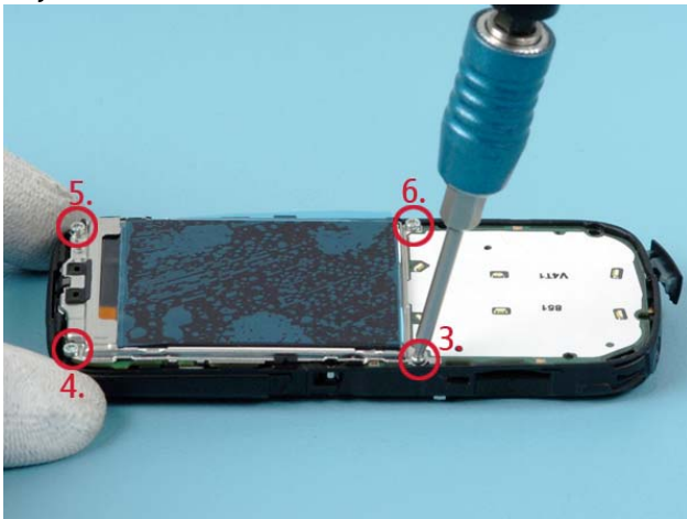
12a) Unscrew the four T6+ screws in the order shown.
