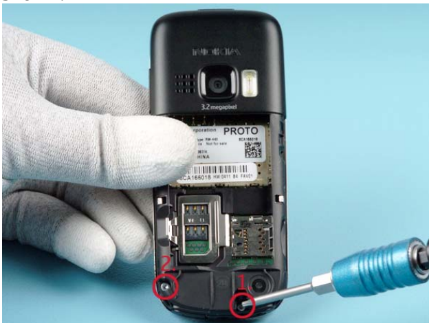
3a) Unscrew the two T6+ screws.
