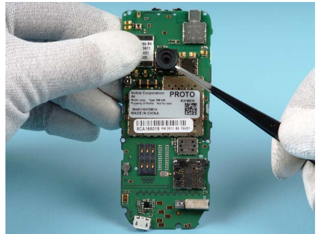
16a) Release the CAMERA GASKET with the tweezers.
