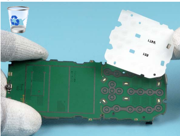
24) Remove the DOMESHEET. Do not use this part again.
