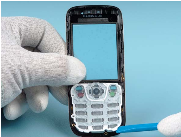
10) Use the SS-93 tool to release the KEYMAT ASSY.
