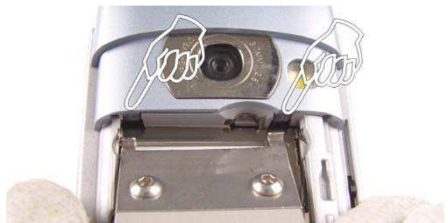
3.) Place the SS-68 into the openings.
