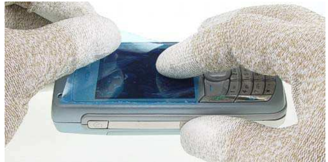
1.) Protect the window with a film.
