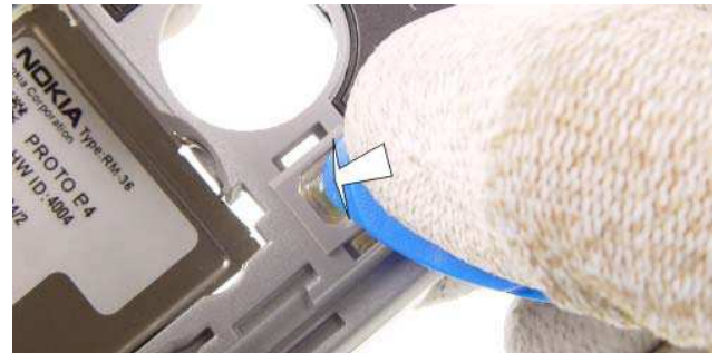
35.) Push out the LED Flash with SRT-6.
