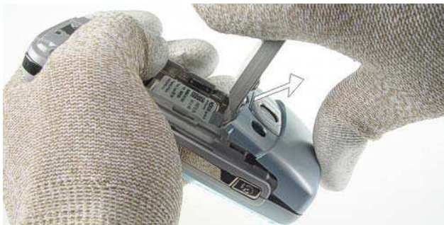
4.) Pull up the Antenna Cover carefully.
