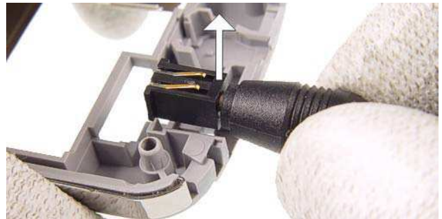
29.) Use the DC plug when removing the DC-Jack .
