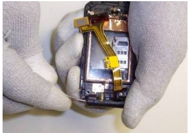
26) Insert the SS-6 Hinge opening tool into the hole in the right hinge.
