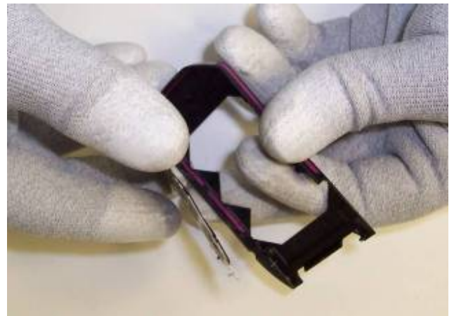
4) Separate the keymat from the C-cover.
