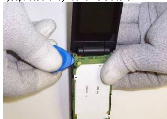
6) Use SRT-6 to separate the PWB from flex conn.
