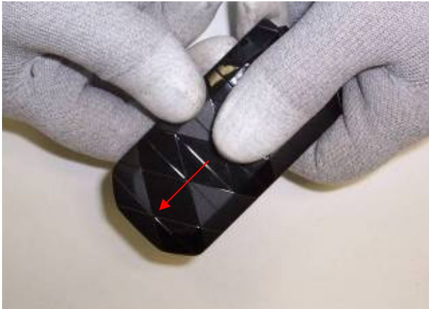
1) Slide the battery cover back and remove it.
