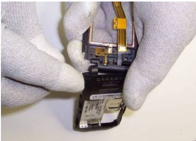
27) Compress the hinge spring and lift to separate it.
