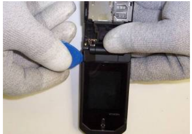
14) Use SRT-6 to remove the right screw cover.
