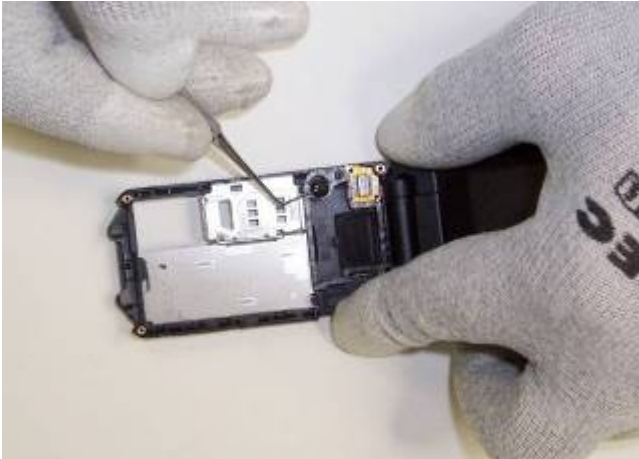
9) Use the dental tool to remove the microphone.
