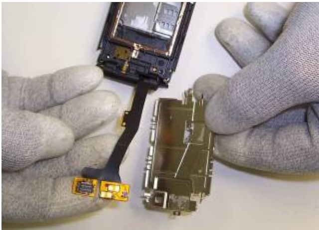
25) Remove the LCD shielding can.
