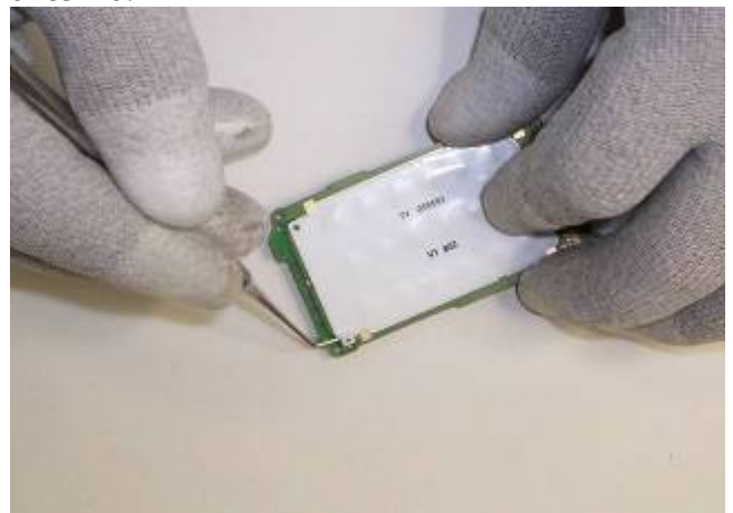
12) Use the dental tool to lift the corner of the dome sheet.
