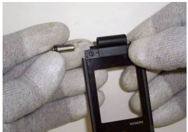
30) Remove the hinge assembly.
