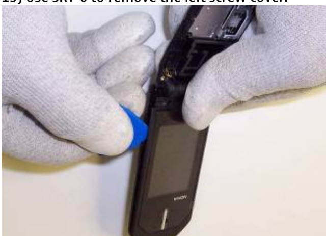
17) Work SRT-6 between and around the A and B covers.
