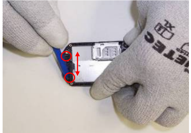
10) Use SS-93 to release the clips holding the antenna.
