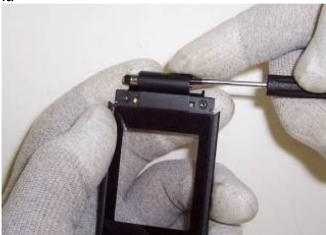
29) Insert a small screwdriver into the B-cover and push out the hinge assembly.
