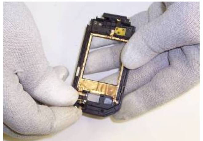
34) Remove the earpiece speaker. The disassembly is completed.
