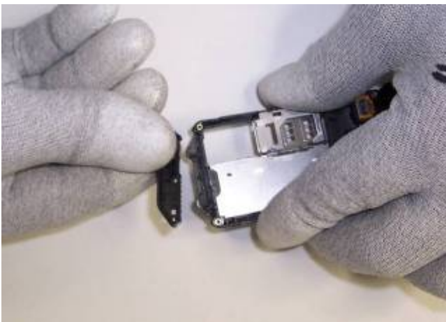
11) Remove the antenna assembly.
