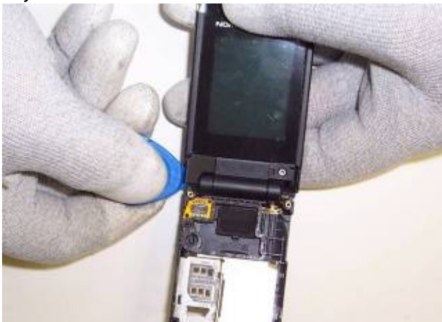
15) Use SRT-6 to remove the left screw cover.
