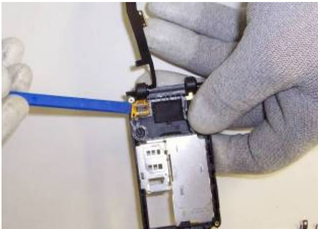
31) Carefully work SS-93 under the UI flex connector and free the hinge flex cable assembly.
