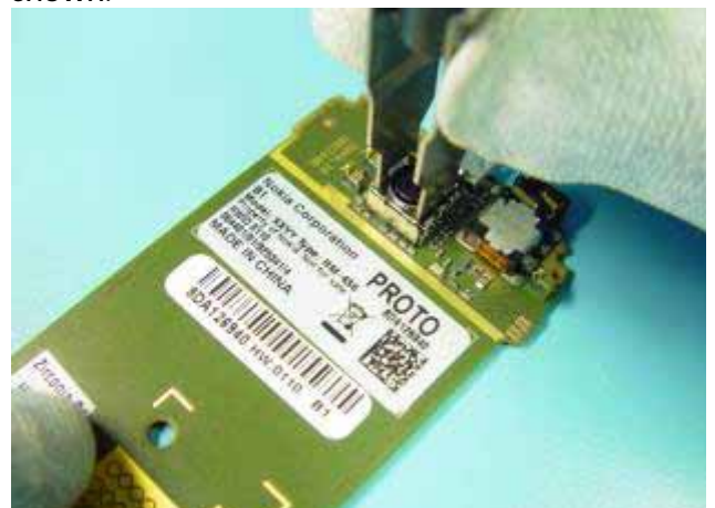
24) Use the camera removal tool SS-88 to release the CAMERA.
