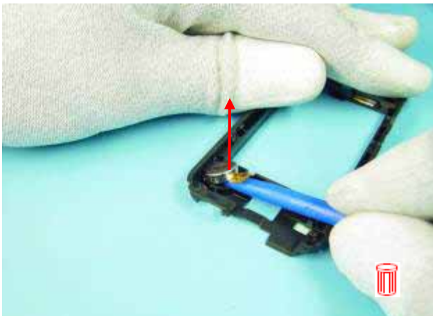
19) Use the SS-93 to lever out the VIBRA MOTOR as shown in the picture. Discard the VIBRA MOTOR.
