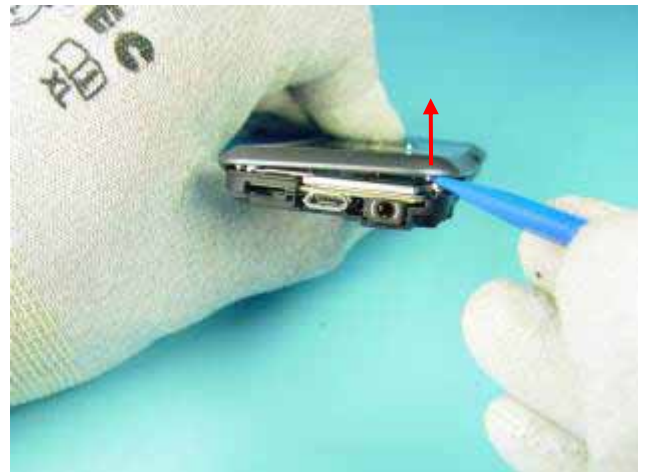
8) Use the SS-93 to detach the A-COVER on the top side.
