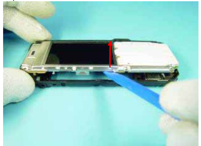
14) Use the SS-93 to lever out the PWB inclusive DISPLAY and UI SHIELD ASSY.
