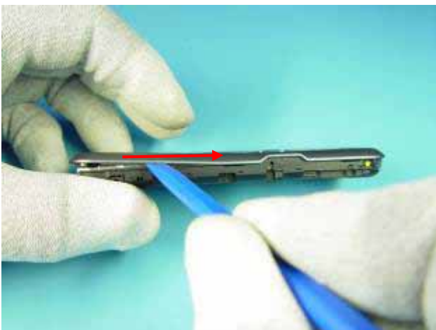
9) Slide the SS-93 along the side walls.
