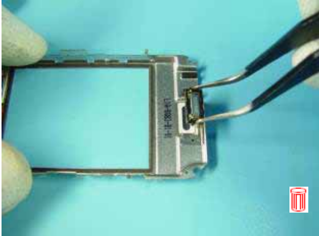
27) Remove the EARPIECE from the UI SHIELD ASSY. Discard the EARPIECE.
