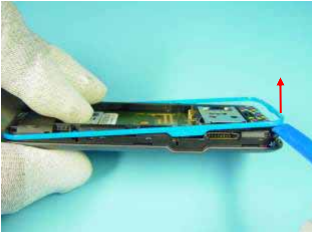
5) Use the SS-93 to detach the SIDE TRIM on the bottom side.
