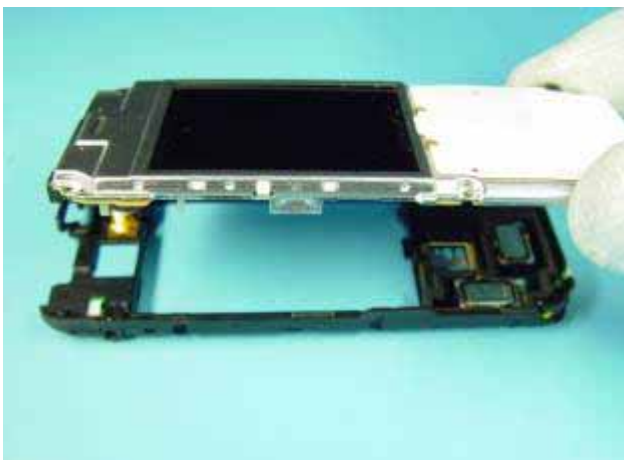
15) Separate the parts from the B-COVER ASSY.
