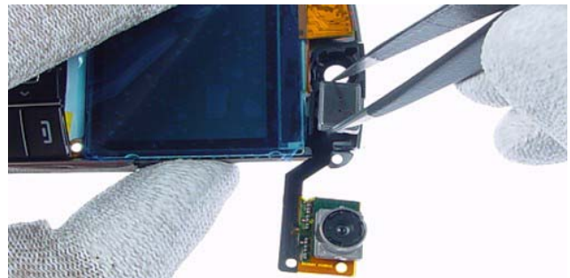
22.) Remove the Earpiece with tweezers.
