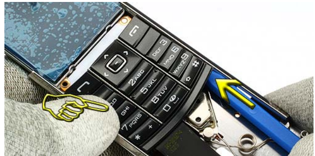
26.) Move the SS-93 along the right edge and fix the Keymat on the left side with your thumb...
