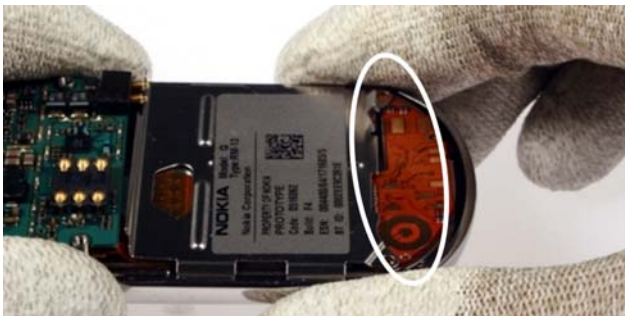
11.) Pull up the A-Cover . Mind the Flex foil's components.
