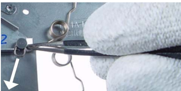
31.) Release the Springs from the middle pin first.
