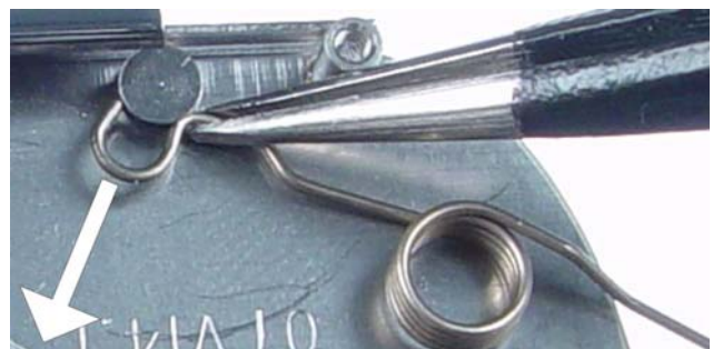
32.) Release the end loop of the Springs .
