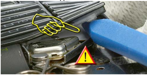
25.) Make sure that the SS-93 is moved between the Keymat and the Domesheet .
