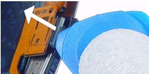
21.) Carefully lever out the Camera Module with the SRT-6 .
