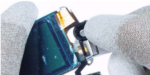
23.) Pull up the Camera Housing .
