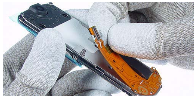
14.) Peel of the Bottom Flex carefully.
