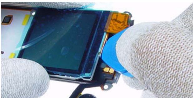
29.) Carefully lift up the Main Flex .
