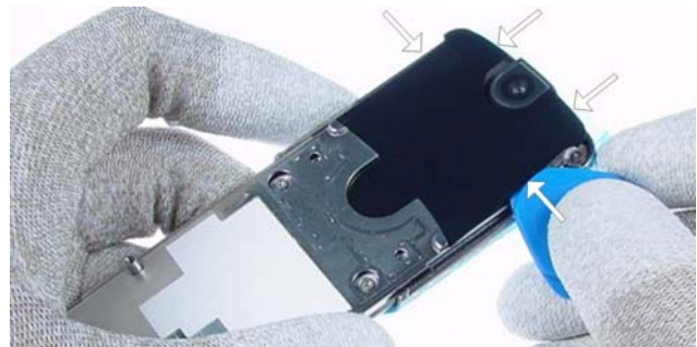
16.) Once released, the Backplate can't be reused again.
