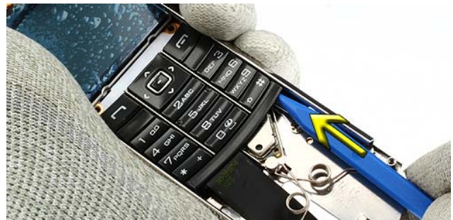
24.) Lever out the Keymat with the SS-93.
