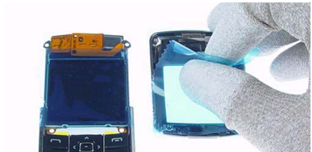
20.) Protect the inner side window and the LCD with a plastic film.
