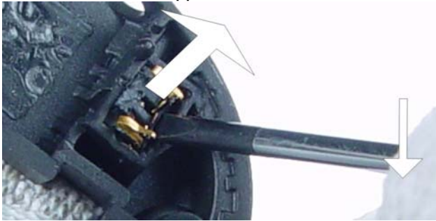
9.) Once removed, the Microphone can't be reused again.
