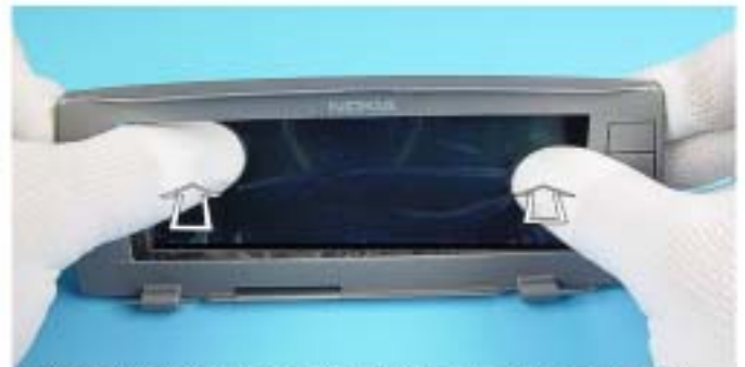
18.) The PDA LCD MODULE is attached with an adhesive tape to the C-COVER. Press out the LCD MODULE slowly and the adhesive will peel away.
