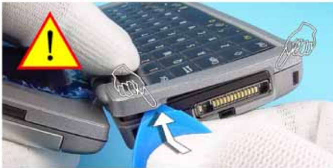
5.) Carefully open the snaps by using the SRT-6.
