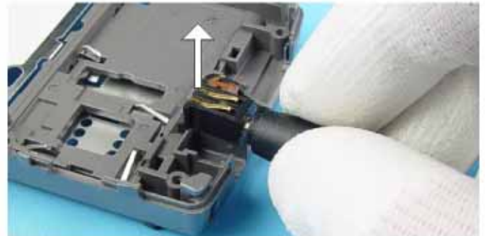
21.) Remove the DC-JACK by using the DC-PLUG.
