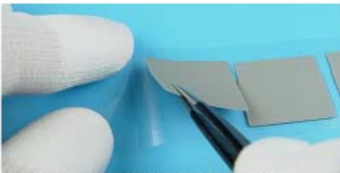
3.) Take the new FLEX COVER by using tweezers...
