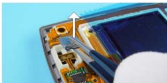
9.) Tweezers can be used to remove the EARPIECE.
