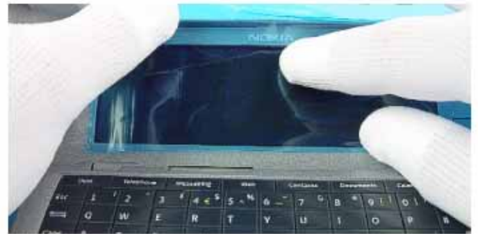
4.) Fit protective film to the PDA LCD MODULE.
