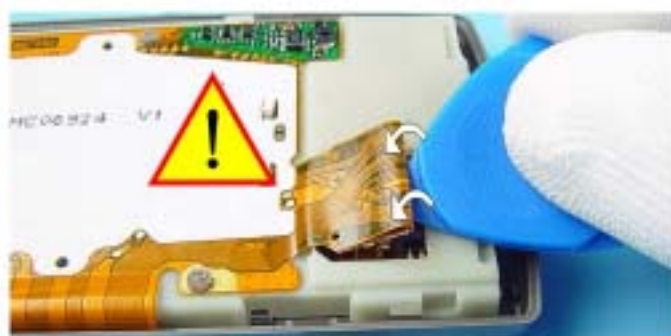
14.) Open the connector by using the SRT-6.
