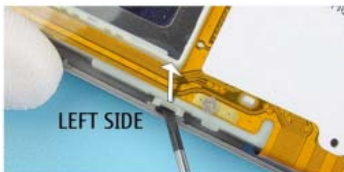
15.) Use a slotted screwdriver as a lever to open the clip.
