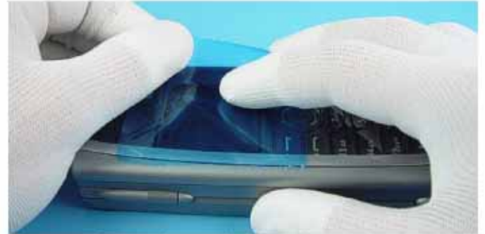
2.) Protect the Window with plastic film.
