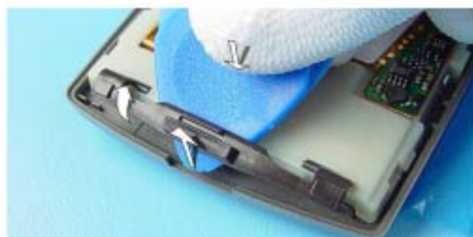
12.) Use the SRT-6 as a lever to open the A-COVER LOCKING.
