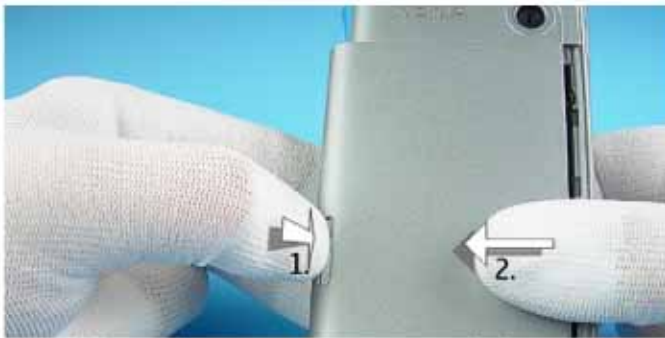
3.) Push down the BATTERY COVER LATCH before opening the BATTERY COVER.
