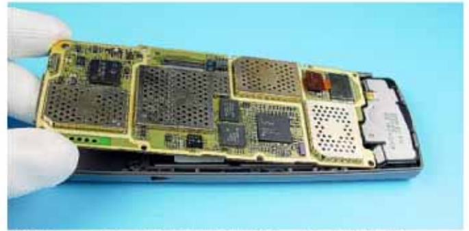
17.) Remove the ENGINE MODULE from the B-COVER.
