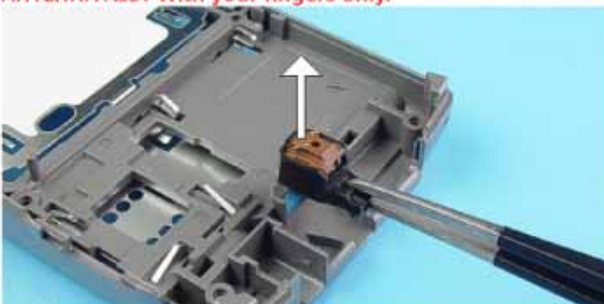
22.) Remove the MICROPHONE with tweezers.
