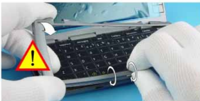
7.) Bend the left side of the KEYPAD FRAME carefully and unlock the snaps as shown.
