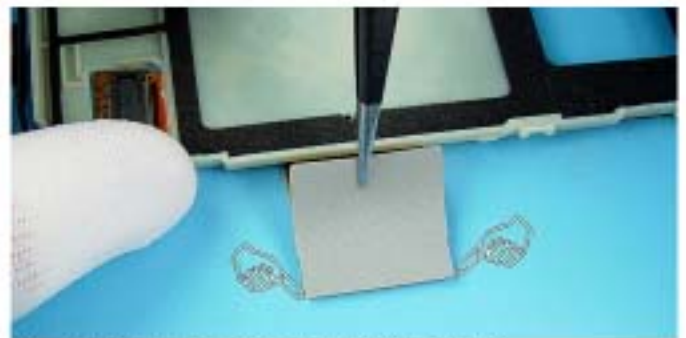
4.) ... and place it on the UI-FLEXFOIL exactly.
