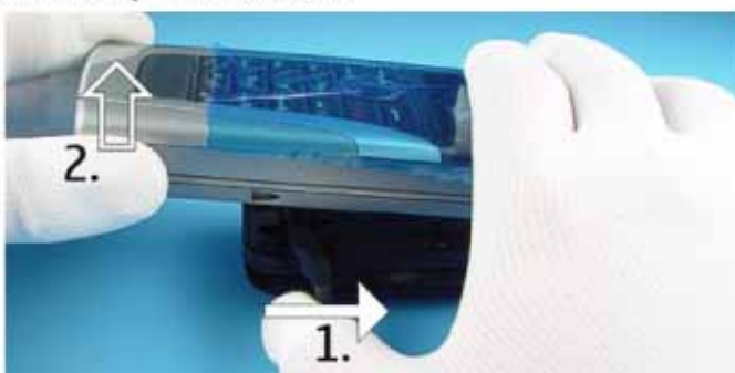
3.) First unlock the FLASH ADAPTER and then lift the bottom side of the device.
