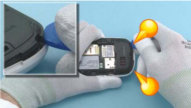
5) Use the SRT-6 to release the B-COVER from the A-COVER, first from the bottom side corners.
