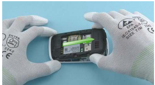
8) Remove the B-COVER including the ENGINE BOARD by lifting it up from the bottom side.
