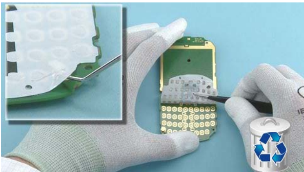
25) Release one corner of the DOMESHEET with the dental tool and peel off the DOMESHEET with tweezers. Do not use it again. Discard it.
