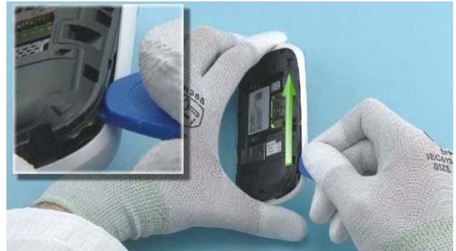
6) Slide the SRT-6 to the direction shown to release the left side of the B-COVER.
