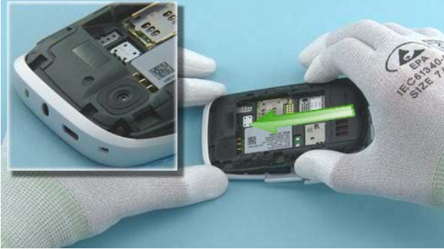
7) Assemble the B-COVER to the A-COVER top side first.
