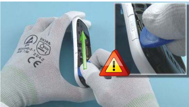
7) Slide the SRT-6 to the direction shown to release the right side of the B-COVER. Be careful with the SD DOOR and the SIM2 DOOR.
