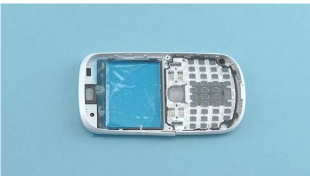
9) Protect the other side of the A-COVER with protective film.
