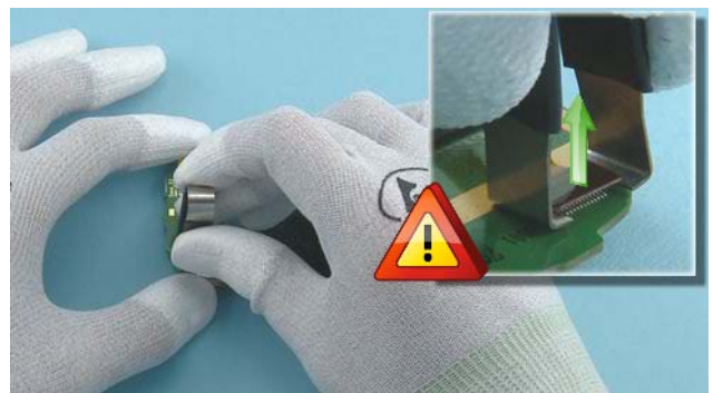
16) Open the DISPLAY connector with the SS-34 flex opening tool. Be careful not to damage the connector.
