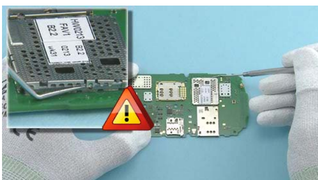
21) Release the BB SHIELDING LID with tweezers. Be careful not to injure yourself or damage any components nearby with the sharp end of the dental tool.
