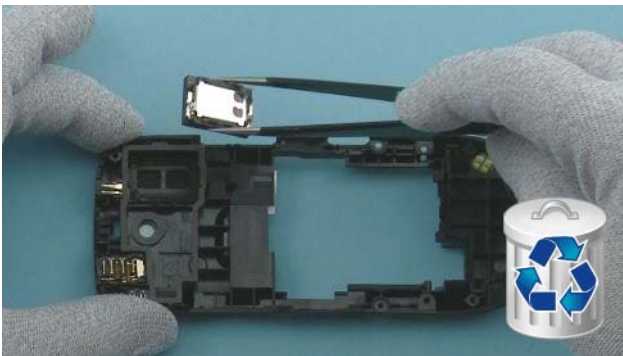
29) Remove the IHF SPEAKER with tweezers Do not use it again. Discard it.
