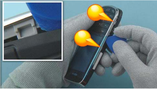
7) Use the SRT-6 to release the snaps holding the A-COVER.
