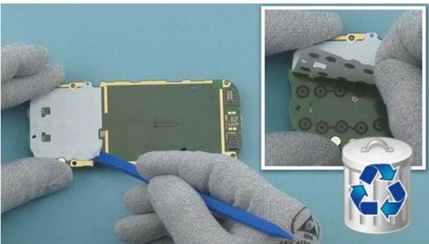
23) Release one corner of the DOMESHEET with the SS-93 and then peel it off with fingers. Do not use it again.
