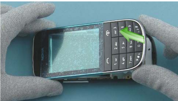
9) To remove the A-COVER, first lift up the bottom end of the A-COVER and then release the top end of the cover.
