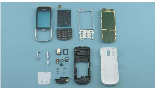
35) Now the Nokia 220/2020 and 203/2030 disassembly procedure is complete.
