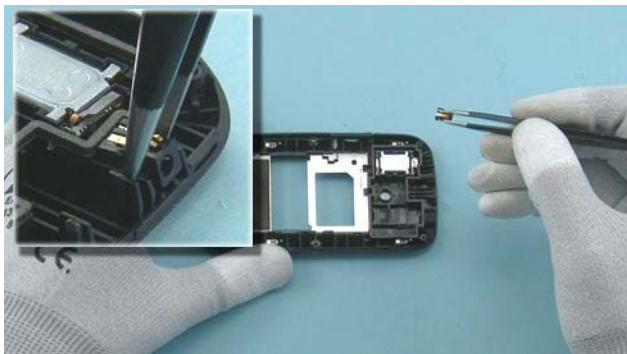
35) Remove the DC JACK with tweezers.
