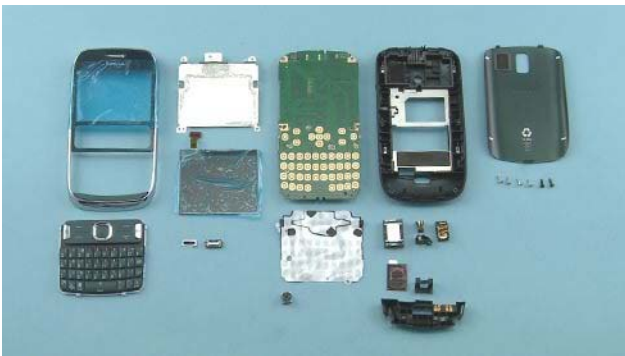
39) Now the Nokia Asha 302 disassembly procedure is complete.
