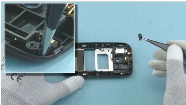
33) Remove the BT/WLAN ANTENNA with tweezers.
