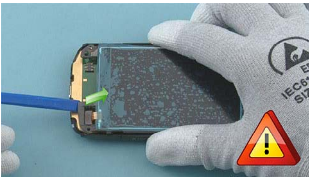
17) Use the SS-93 to carefully lift up the UI FRAME a little bit to gain access to the DISPLAY CONNECTOR.
