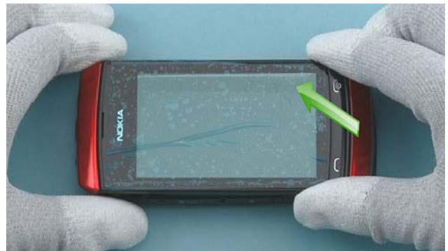
10) To remove the A-COVER, first lift up the bottom end of the A-COVER and then release the top end of the cover.
