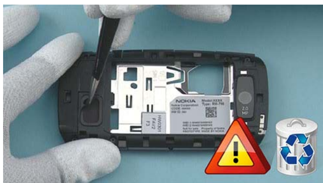
35) Use the tweezers to carefully remove the SPEAKER GASKET with MESH. Do not use it again. Make sure there are no adhesive residues left in the slot.
