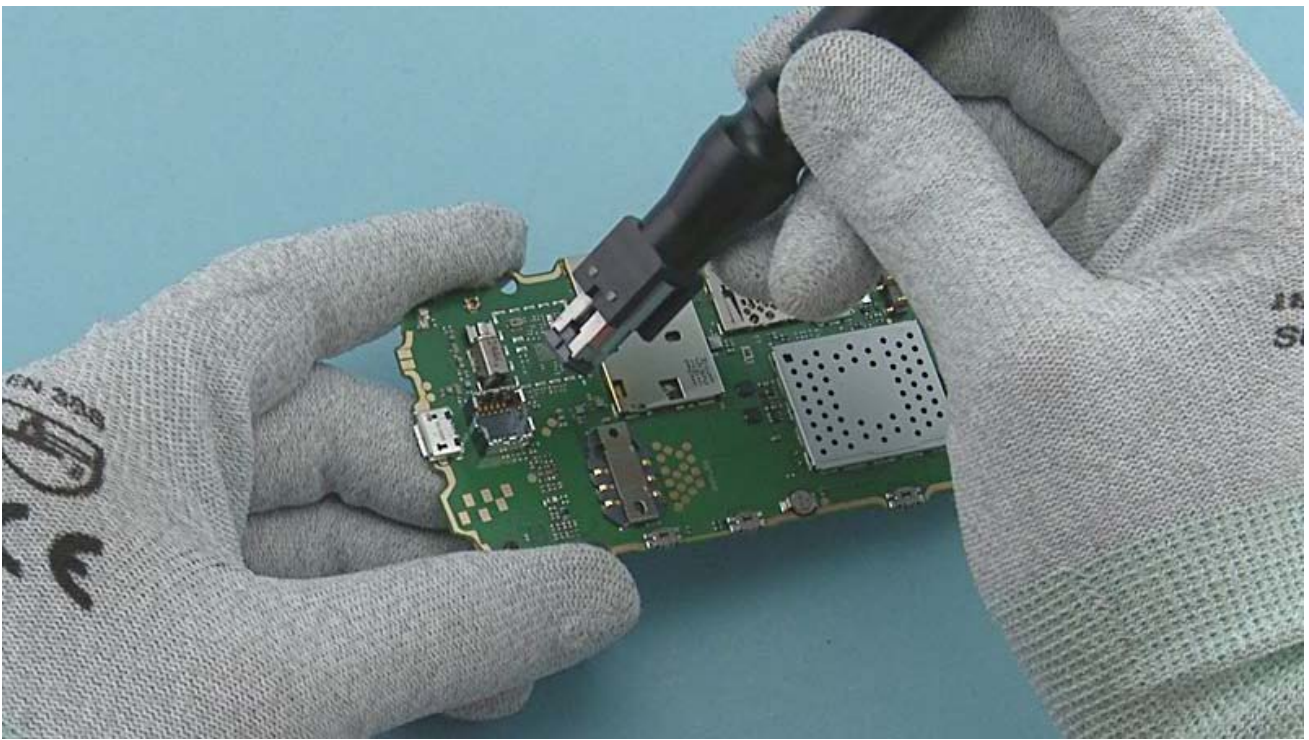
Lift up the SS-276 and remove the CAMERA.
