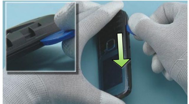
8) Release the other side of the A-COVER from the D-COVER by sliding the SRT-6 to direction shown.
