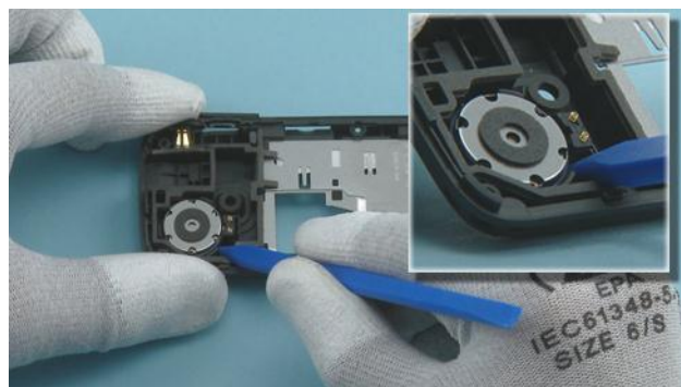
20) Use the sharp end of the SS-93 to release the EARPIECE / SPEAKER / VIBRA.
