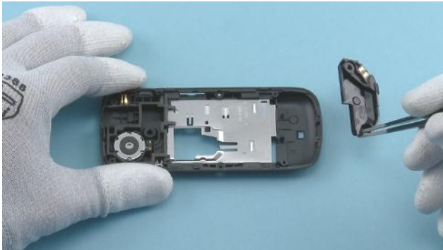
25) Remove the ANTENNA MODULE with the tweezers.
