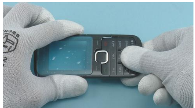
12) Push down to release the KEYMAT.
