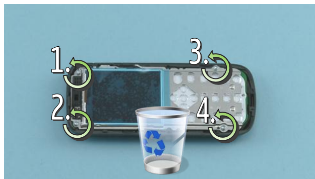
14) Unscrew the four Torx+ size 6 screws. Do not use them again. Discard them.
