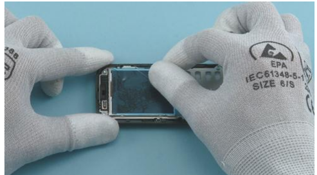
10) Protect the DISPLAY with the protective film.
