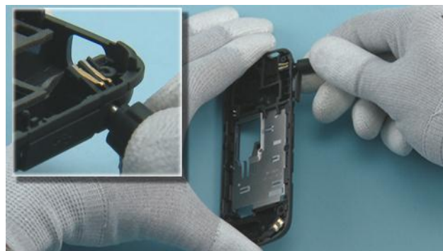
22) Release the DC JACK with the DC plug.
