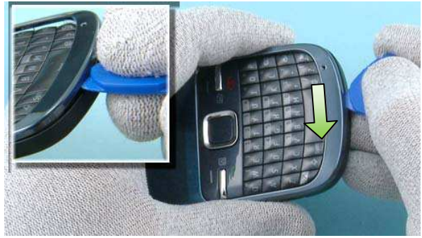
8) Then release the clips on the bottom side.
