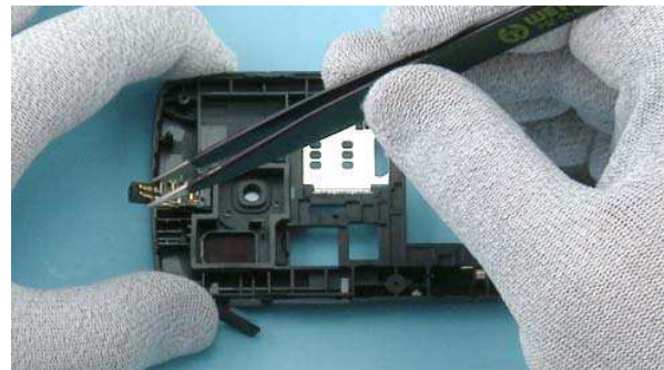
24) Remove the DC JACK with the tweezers.
