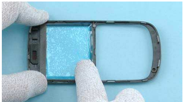
12) Protect also the other side of the A-COVER window with a protective film.
