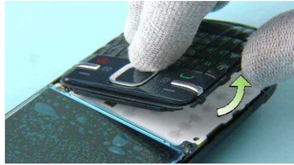
14) Then lift up the KEYMAT ASSY from bottom left side.
