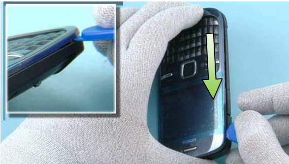
9) Continue to slide the SRT-6 in the direction shown to release the clips on the other side. Start detaching the clips near the release button.
