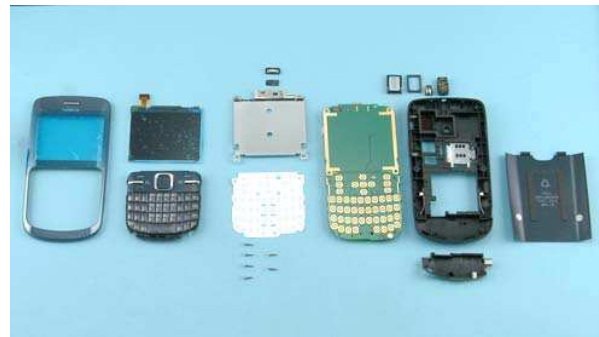
42) Nokia C3-00 disassembly is now complete.
