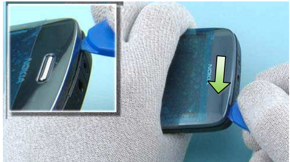
10) Finally release the clips on the top side and remove the A-COVER.
