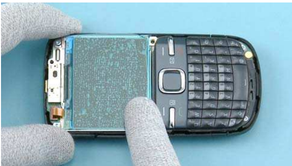
11) Protect the LCD with a protective film.
