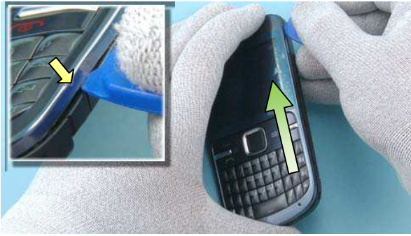
7) Detach the A-COVER by sliding the SRT-6 in the direction shown. Start detaching the clips near the release button.
