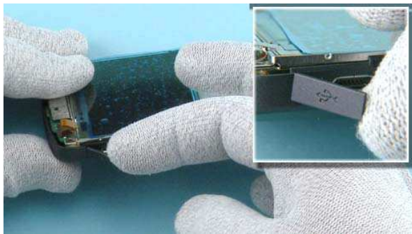
17) To release the engine board, open the USB door.
