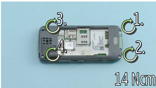
19. Tighten the four TORX+ size 6 screws to the torque of 14 Ncm in the order shown.
