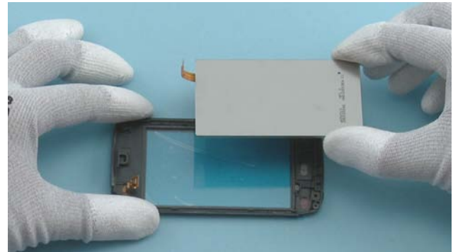
20. Lift the DISPLAY away from the FRONT COVER ASSEMBLY.
