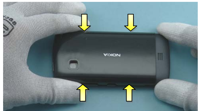
22. Insert the BATTERY and place the BATTERY COVER to its place. Press it gently to lock up the clips.
