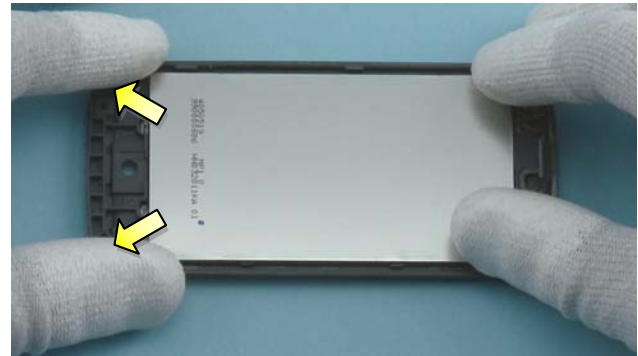
14. Remove the protective films from the DISPLAY and the FRONT COVER. Place the DISPLAY to the FRONT COVER and make sure that it is correctly aligned.
