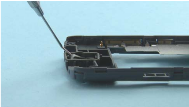
37. Loosen the EARPIECE ADHESIVE with the dental tool.
