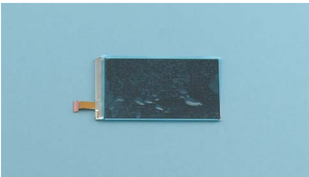
21. Protect the DISPLAY with protective film.
