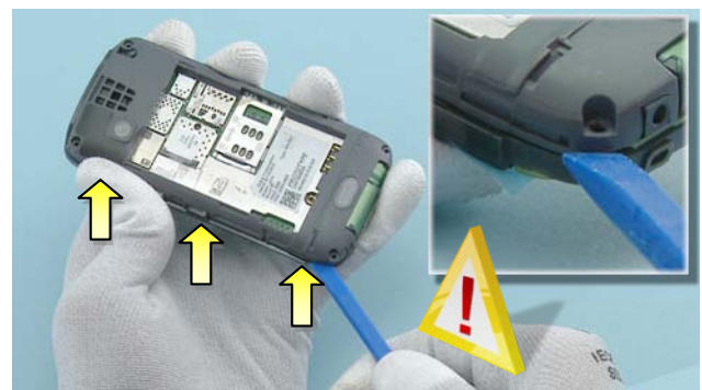
12. Use the SS-93 to detach the three shown clips of the FRONT COVER ASSEMBLY. Be careful not to damage any nearby components.
