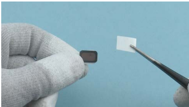
3. Remove the protective film from the EARPIECE ADHESIVE.
