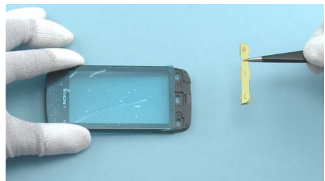
24. Remove the KEYMAT with the tweezers.
