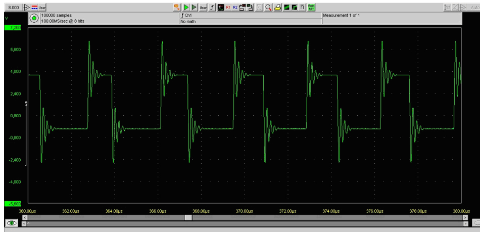
Figure 36 Single-ended output waveform of the Ext_microphone in Int handsfree out loop measurement when speaker is connected (measured at speaker pads). No filter is used.
