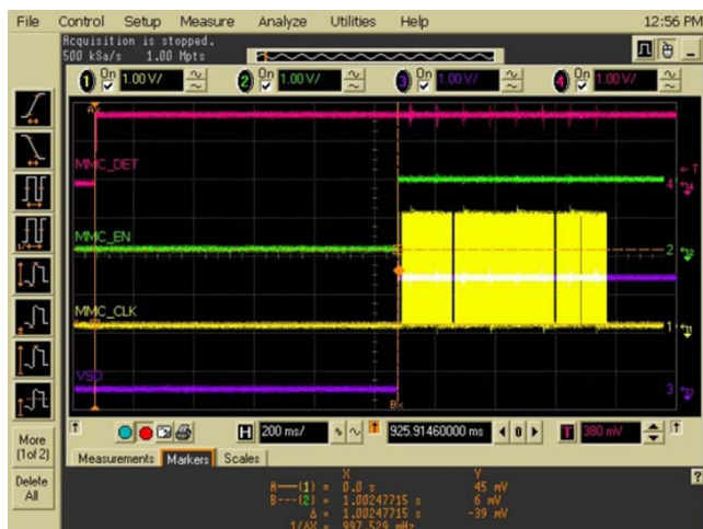
MicroSD interface signals timing when door is closed.
