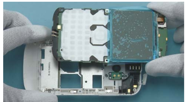
24) Lift up the LIGHT SWAP PWB and remove it.
