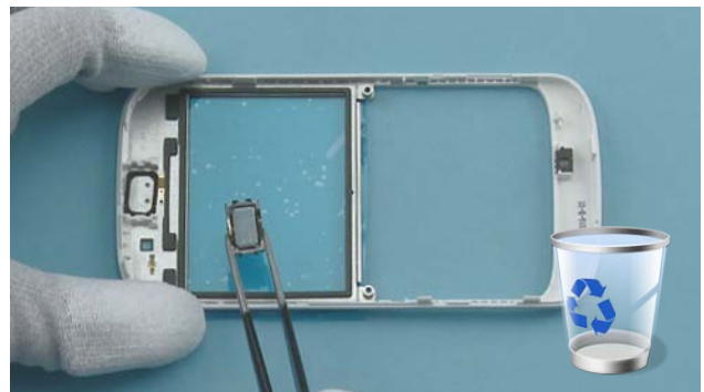
16) Remove the EARPIECE with the tweezers. Do not use it again.
