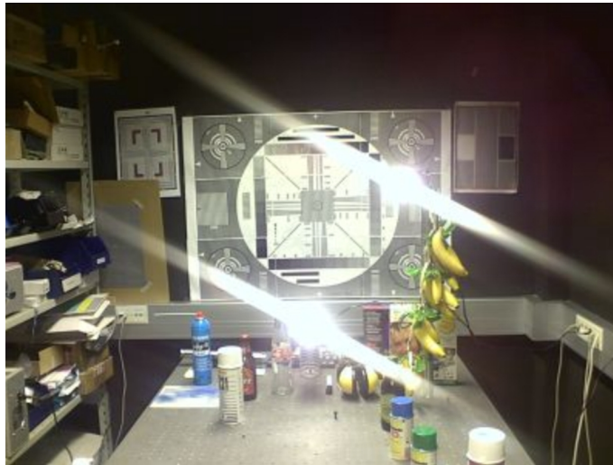
Figure 37 Image of point light sources taken with a dirty (finger print) protective window
