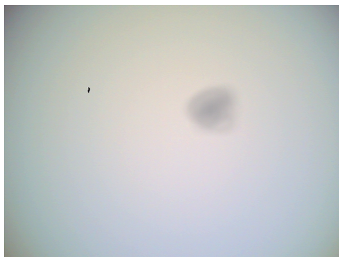
Figure 33 Effects of dust on optical path
