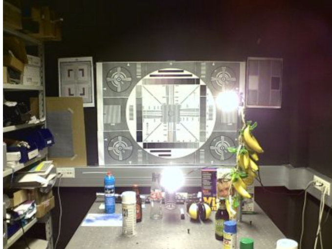
Figure 36 Image of point light sources taken with a clean protective window
