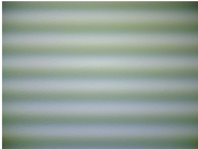
Figure 29 Flicker in an image; object illuminated by strong fluorescent light
