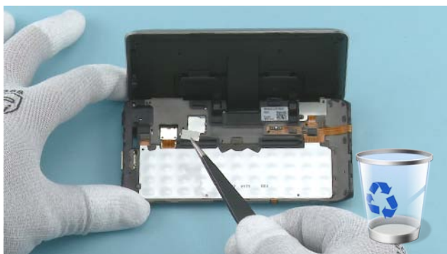
25) Remove the CONNECTOR LOCK PLATE with the tweezers. The CONNECTOR LOCK PLATE cannot be reused. Discard it.
