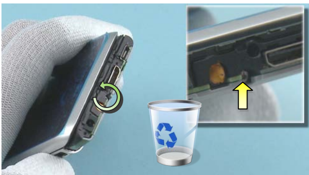
15) Unscrew the shown Torx+ size 4 screw. Do not use it again. Discard it.
