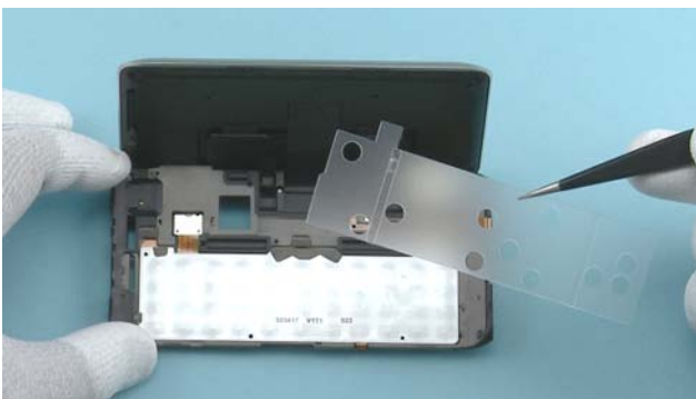
35) Remove the DUMMY KEYMAT with the tweezers and close the device.
