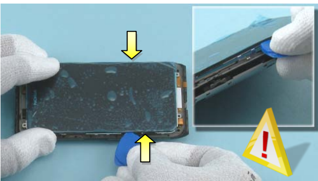
53) Lift up the WINDOW very carefully with the SRT-6 from both sides. Be careful not to damage the WINDOW flex! Note that only the WINDOW has to be lifted. The DISPLAY should remain on its place.
