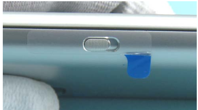
74) Remove the lock key protective film.
