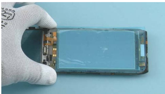
55) Protect the DISPLAY with protective film.
