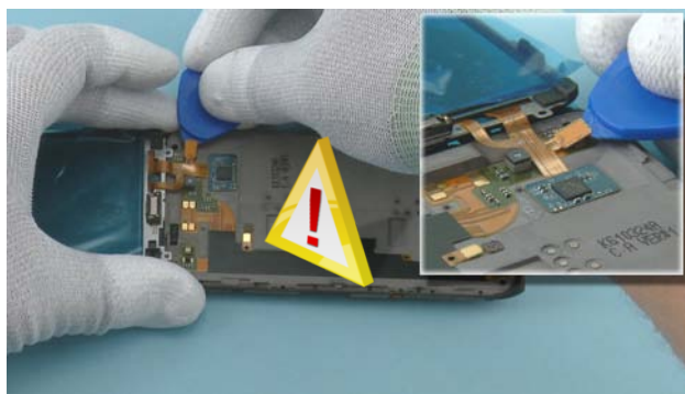
62) Open the WINDOW connector with the SRT-6. Be careful not to damage the connector.
