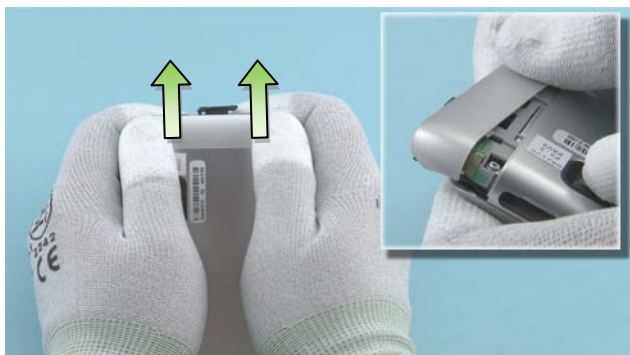
9) Release the TOP END CAP by pushing it to the direction shown.
