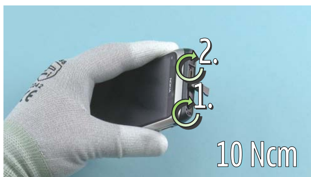
65) Tighten the two TORX + size 4 screws to the torque of 10 Ncm in the order shown.
