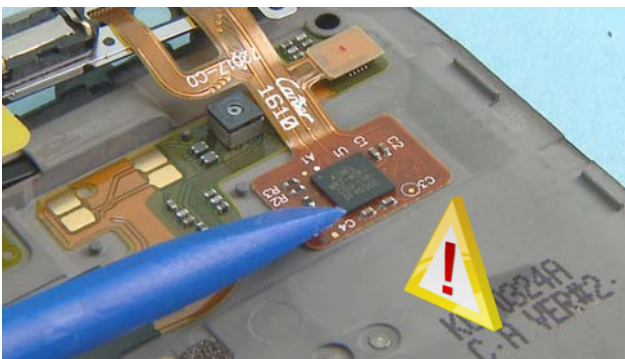
17) Attach the WINDOW flex adhesive by gently pressing with the SS-93. Be careful not to damage the connector or any nearby components.
