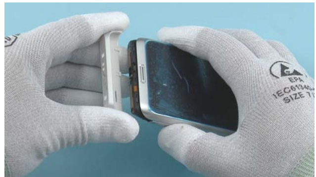
14) Pull out and remove the BOTTOM END CAP.
