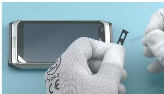
68) Remove the protective film also from the other side.
