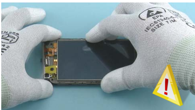
21) Turn around the DISPLAY. Be careful not to damage the DISPLAY flex while turning the DISPLAY.
