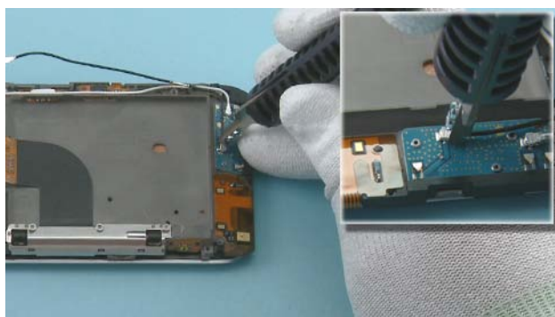
42) Use the SS-231 to release the other end of the BLACK COAX CABLE.
