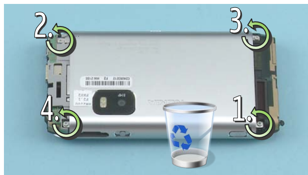
20) Close the device and unscrew the four Torx+ size 4 screws in the order shown. These screws cannot be used again. Discard them.
