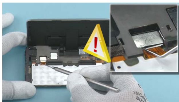
24) Open the device as shown. Release the CONNECTOR LOCK PLATE carefully with the dental tool. Be careful not to injure yourself or the connector under the CONNECTOR LOCK PLATE with the sharp end of the dental tool!
