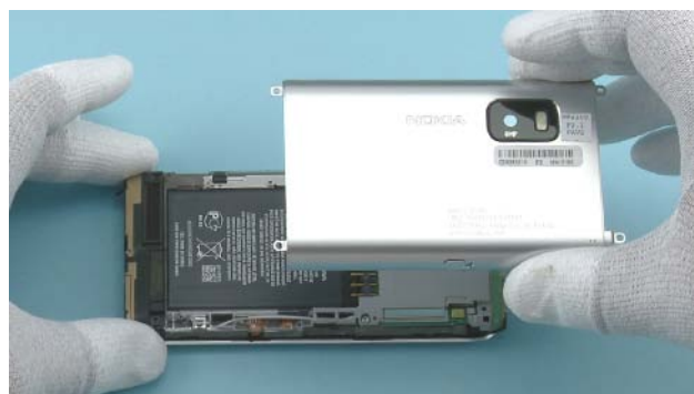
22) Lift up and remove the BACK COVER.
