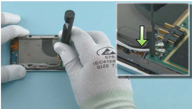
33) Use the RF connector tool SS-231 to release the two coax cables. First place the tool on top of the cable.
