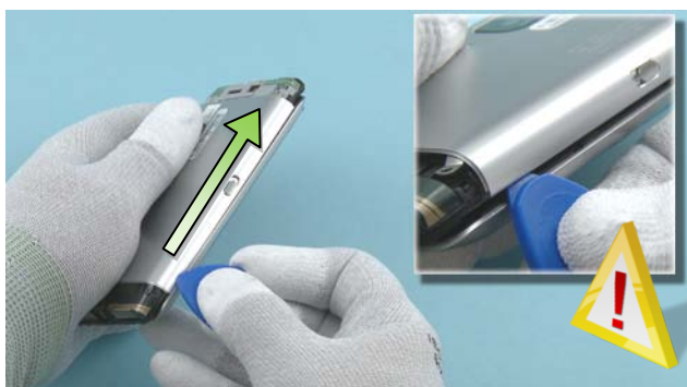
21) To release the BACK COVER, insert the SRT-6 between the BACK COVER and the BASE CHASSIS. Then slide the SRT-6 to the direction shown. Do this ONLY on LOCK KEY side!
