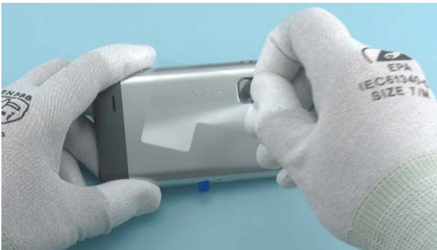
73) Remove the protective film from the back cover.
