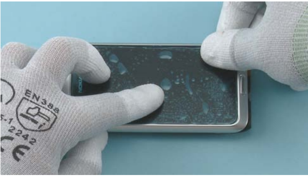
49) Close the device. Release the LID FRAME by lifting up from one of its corners.
