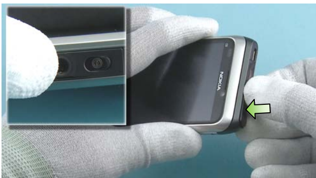
69) Place the TOP END DECO as shown. Push the TOP END DECO to lock it into its place.
