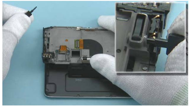
32) Pull out and remove the HINGE PIN to release the BASE CHASSIS ASSEMBLY.
