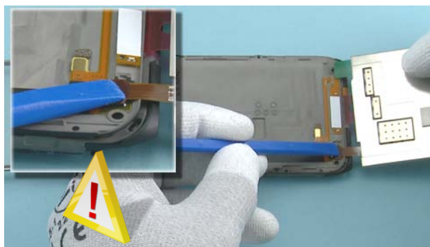
20) Connect the DISPLAY connector with the SS-93. Be careful not to damage any nearby components.
