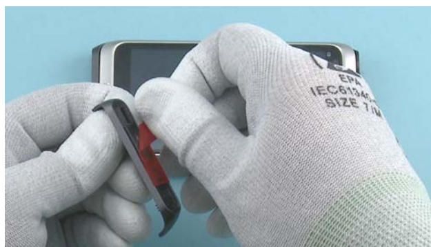
62) Remove the protective film from the TOP END CAP.
