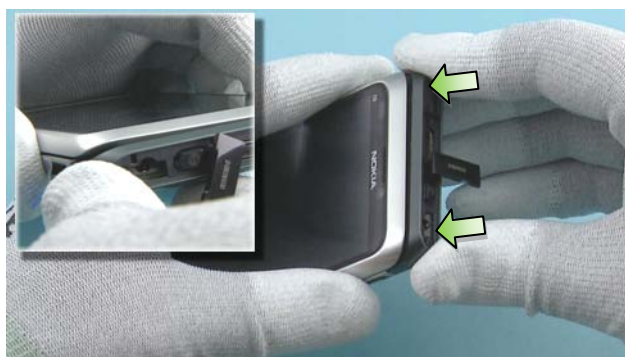
64) Push the TOP END CAP into its place as shown. Make sure the TOP END CAP is correctly in its place and there are no gaps visible.
