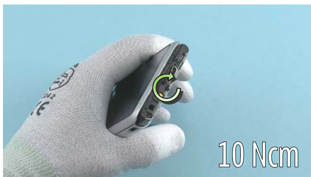
61) Tighten the TORX + size 4 screw to the torque of 10 Ncm.
