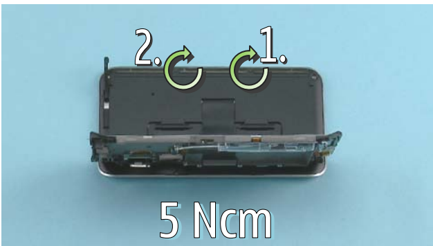
33) Tighten these two TORX + size 4 screws to the torque of 5 Ncm in the order shown.
