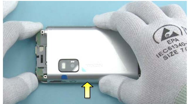
52) Insert the shown side of the BACK COVER into BASE CHASSIS ASSEMBLY.
