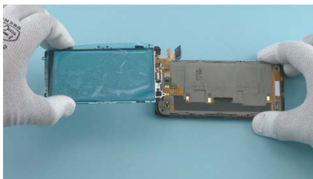
64) The WINDOW can now be separated.
