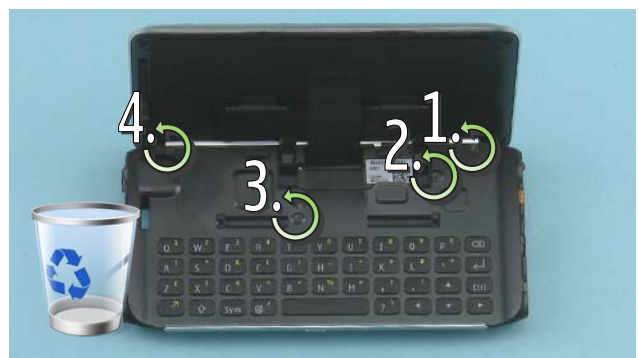
18) Unscrew the four Phillips size 00 screws in the order shown. Do not use them again. Discard them.
