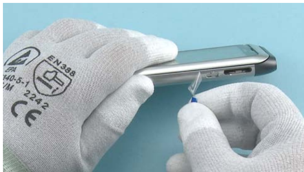
70) Remove the volume key protective film.
