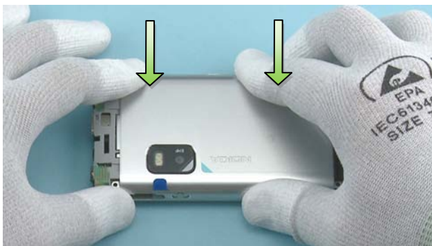
53) Then press from the opposite side to lock the BACK COVER to the BASE CHASSIS ASSEMBLY.
