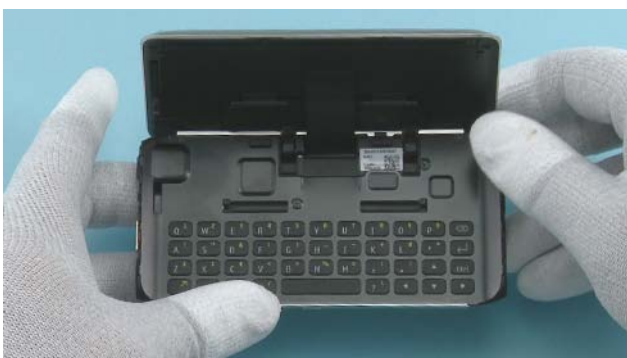
17) Then turn the display part of the device as shown.
