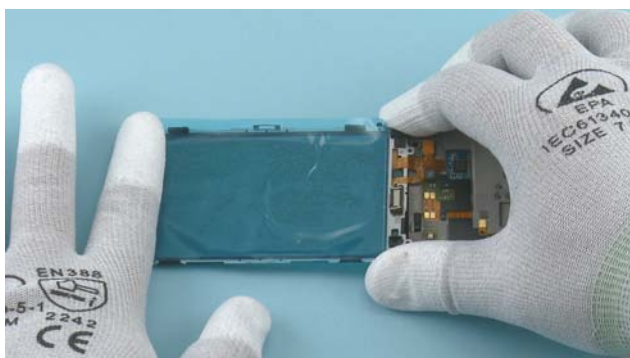
59) Protect the other side of the WINDOW with protective film.
