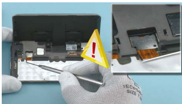
26) Open the QWERTY FLEX MODULE connector with the dental tool. Be careful not to damage the connector or any nearby components!
