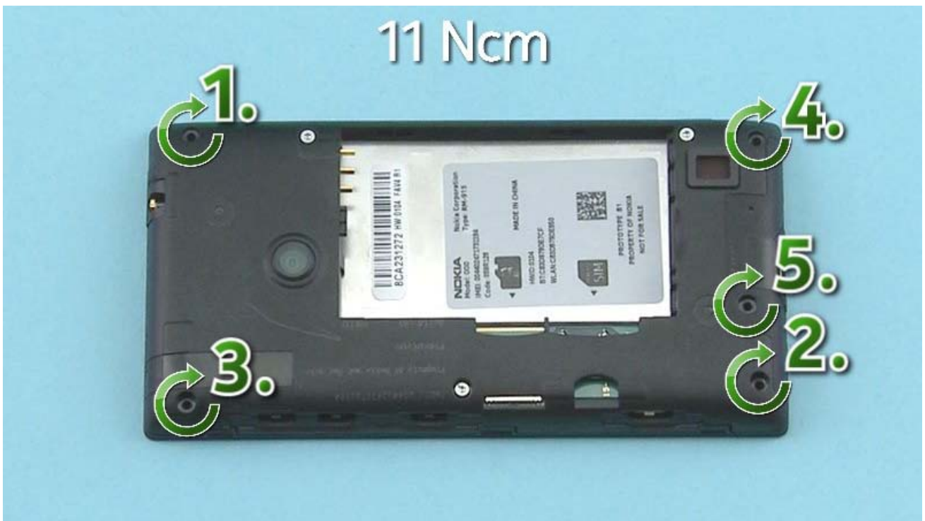
6) Fasten the five Torx+ size 4 screws in the order shown to the torque of 11 Ncm.
