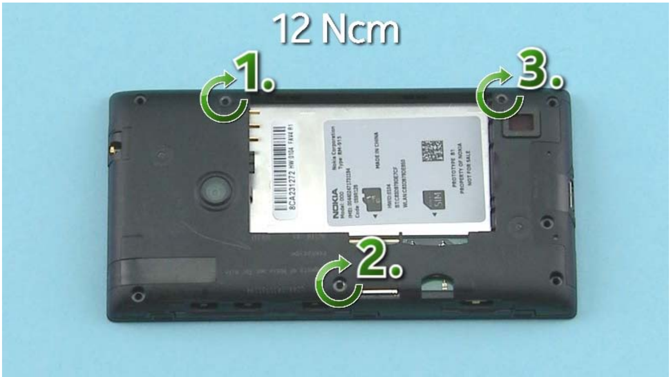
5) Fasten the three Torx+ size 4 screws in the order shown to the torque of 12 Ncm.
