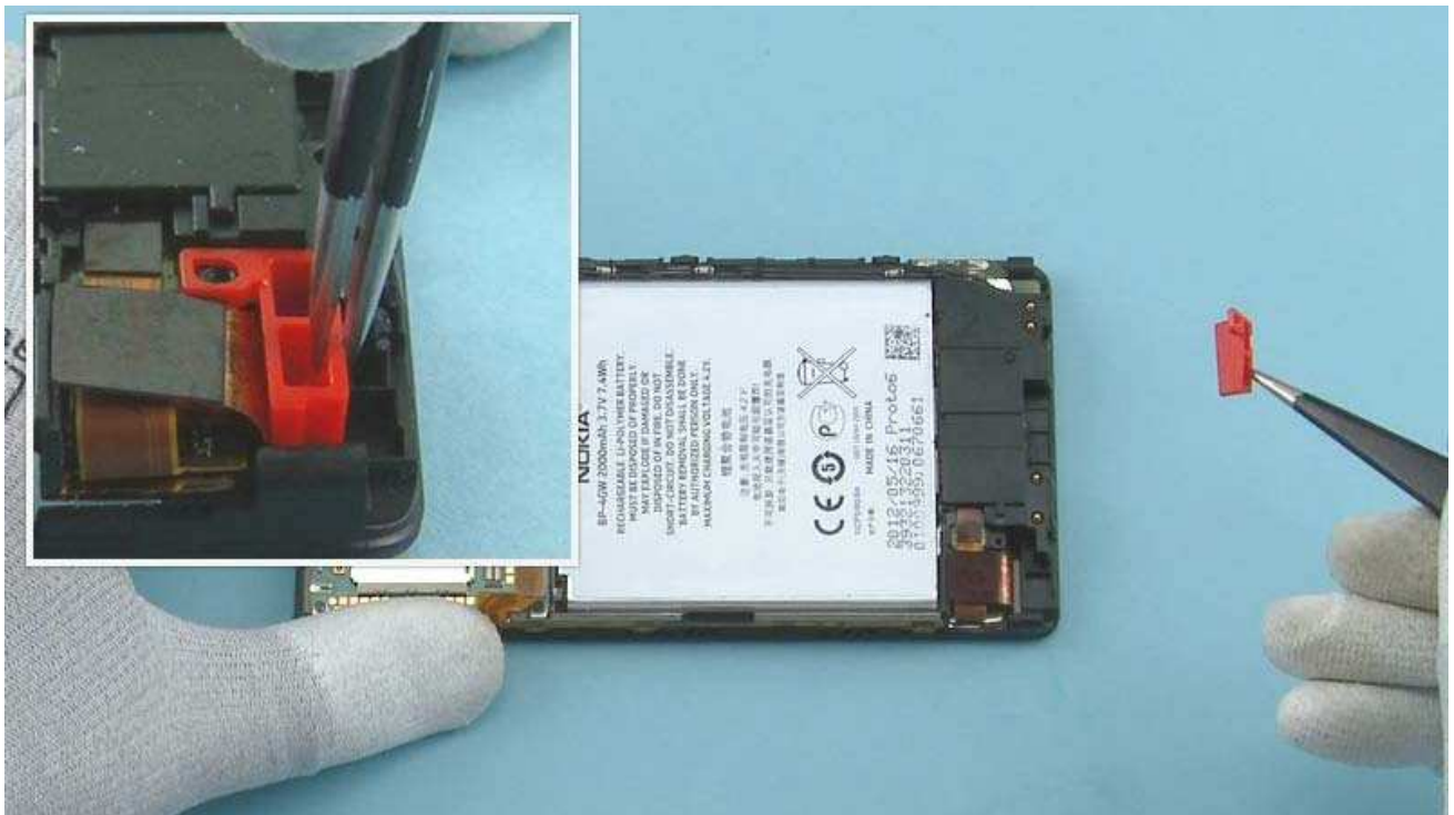
Remove the BATTERY SUPPORT with tweezers.
