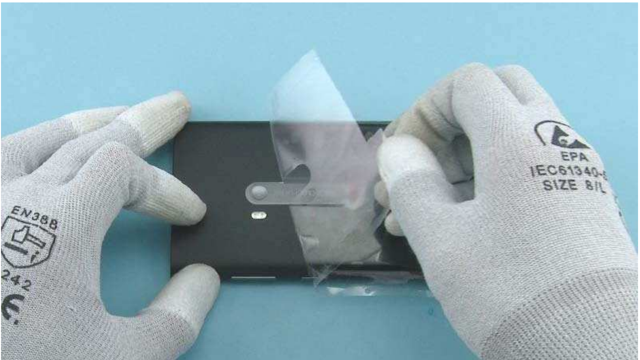
Remove the UNIBODY ASSEMBLY protective film.
