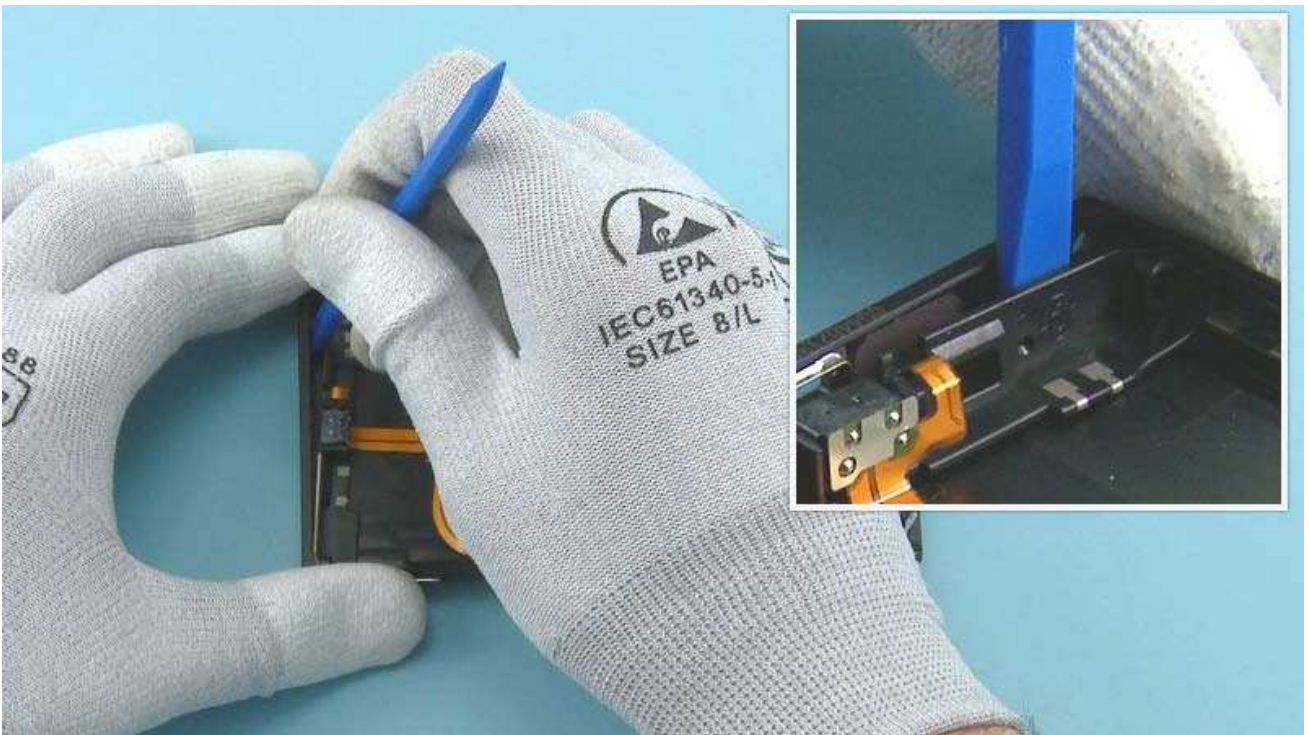
To remove the MAIN ANTENNA first push the other side out slightly with the SS-93.
