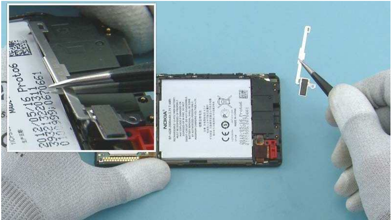
Remove the BATTERY HOLDER with tweezers.
