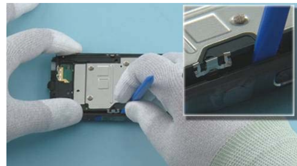
30) Use the SS-93 to spread the sides of the BODY ASSY and push down the ENGINE CHASSIS ASSY to lock the springs.
