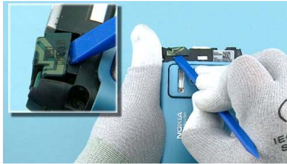
25) Release the COMBO ANTENNA with the SS-93.
