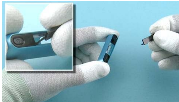
13) Pull out and remove the HDMI HATCH.
