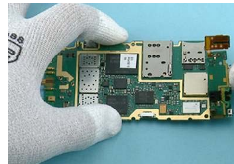
40) Turn over the SUB PWB. Be careful not to damage the flex!
