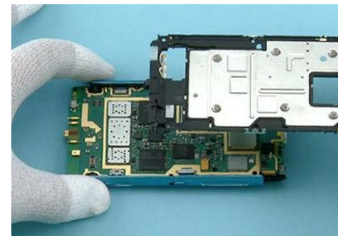
28) Lift up and remove the ENGINE CHASSIS
