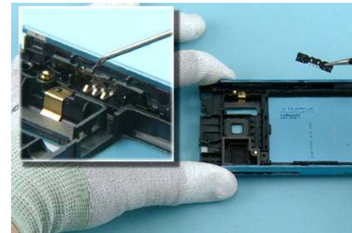
50) Release the SIDE SWITCH with the dental forceps. Remove it with the tweezers.
