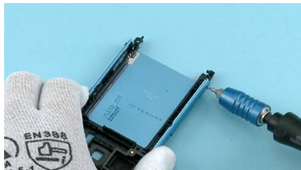
51) Unscrew the Torx+ size 4 screw to release the FIXING NUT.
