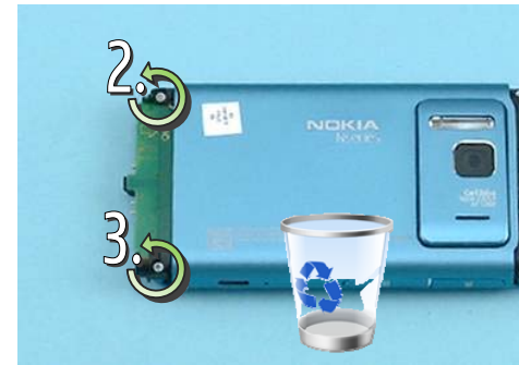
14) Unscrew the four Torx+ size 5 screws in order shown. These screws cannot be reused. Discard them.
