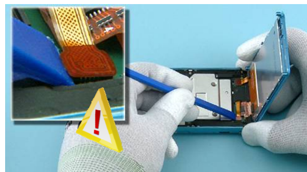
18) Use the SS-93 to open the WINDOW ASSY CONNECTOR. Be careful not to damage the connector or components nearby!
