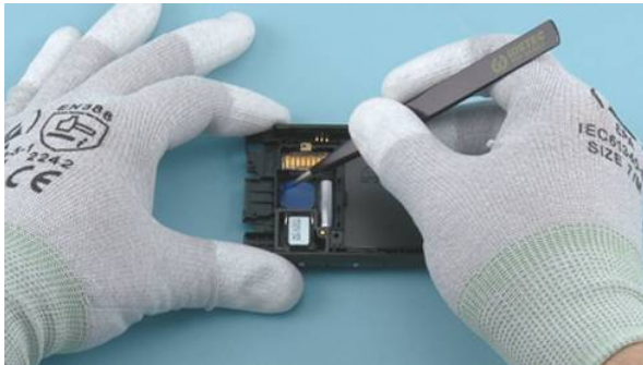
19) Remove the camera lens protective film with the tweezers.
