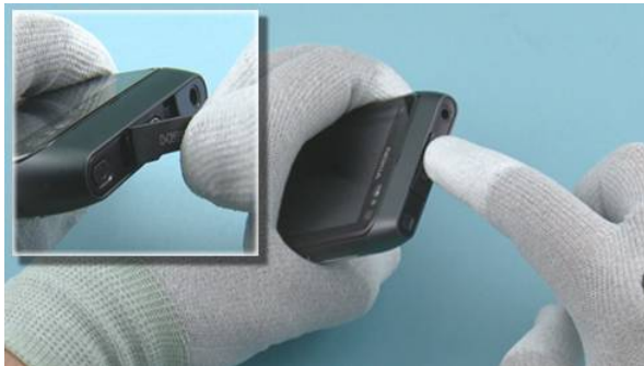
43) Close the HDMI HATCH and check that the TOP COVER edges are attached properly.
