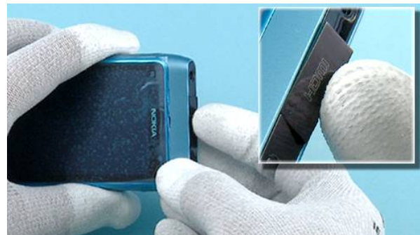
10) Open the HDMI HATCH.
