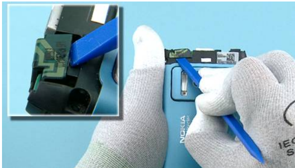
25) Release the COMBO ANTENNA with the SS-93.
