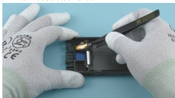
12) Place the FLASH MODULE with the tweezers.
