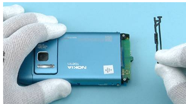
8) Now the BATTERY LID can be removed.
