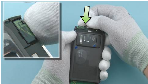
33) Push the COMBO ANTENNA into place.
