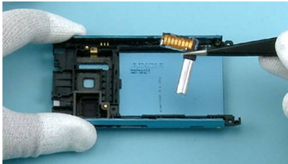
49) Remove the FLASH MODULE with the tweezers.
