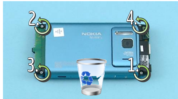
14) Unscrew the four Torx+ size 5 screws in the order shown. These screws cannot be used again. Discard them.
