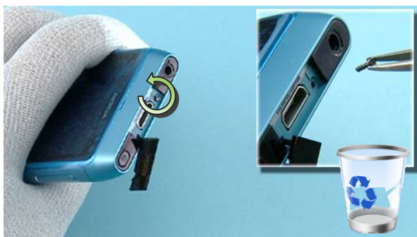
11) Unscrew the Torx+ size 5 screw. Do not use it again. Discard it.
