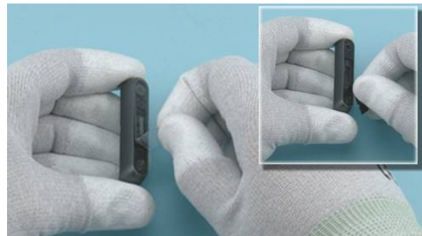
40) Remove the protective film from the TOP COVER and open the HDMI HATCH.
