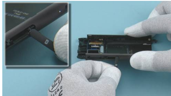
14) Insert the SIM CARD HATCH fastener into the BODY ASSY cavity. Then press the SIM CARD HATCH into place.
