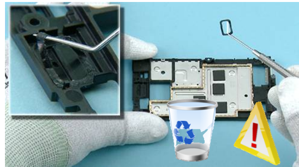
34) Remove the EARPIECE GASKET with the dental tool. Be careful not to injure yourself with the sharp end of the dental tool! The EARPIECE GASKET is not reusable. Discard it.
