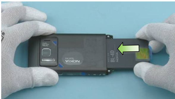
45) Insert the BATTERY as shown.
