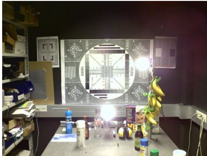
Figure 41 Image of point light sources taken with a clean protective window
