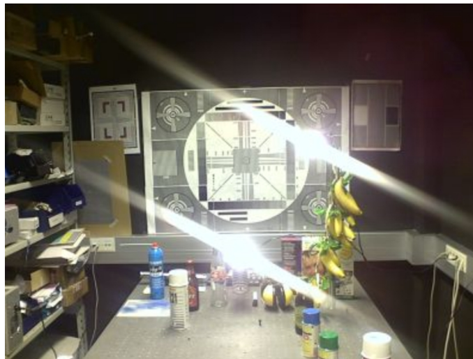
Figure 42 Image of point light sources taken with a dirty (finger print) protective window
