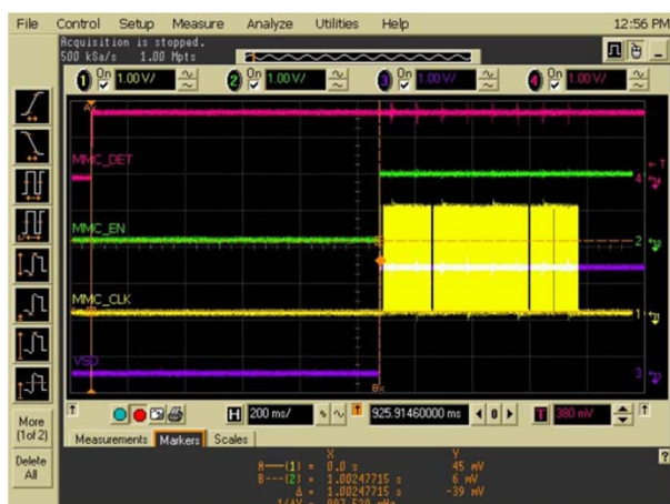
MicroSD interface signals timing when card is inserted.
