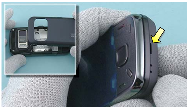
4) Release the BATTERY COVER and remove it.
