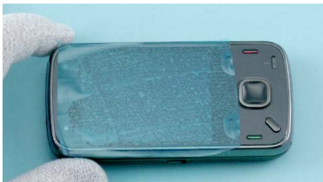
3) Protect the front cover with a protective film.
