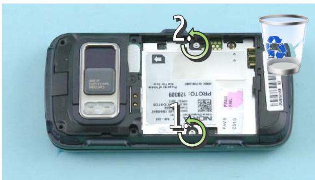
9) Then unscrew these two TORX + size 4 screws in the order shown. Do not use them again.
