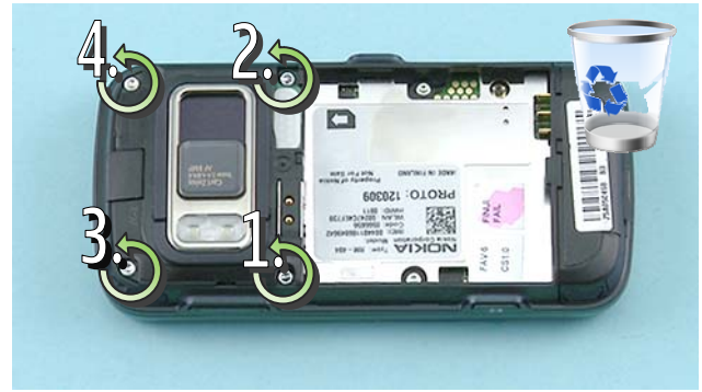
8) Unscrew the four TORX+ size 6 screws in the order shown. Do not use them again.
