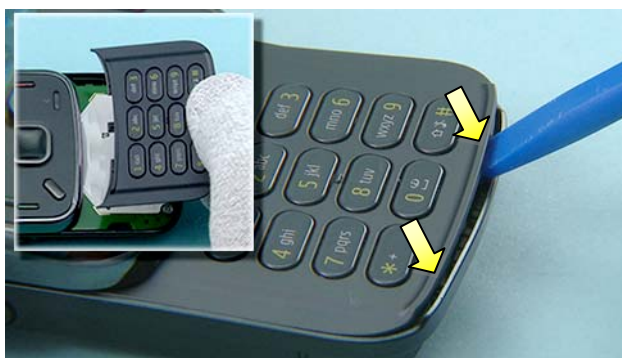
6) Use the SS-93 to release the keymat and remove it by pulling it.
