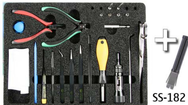
1) You must use the Nokia Standard Toolkit version 2 and the SS-182 camera removal tool.
