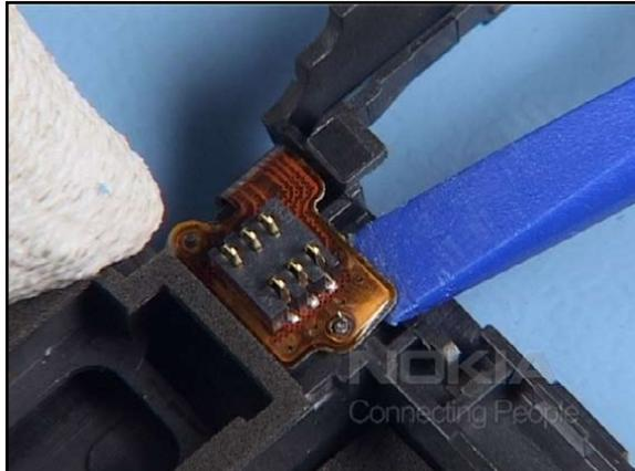
32. Release the flex of the 1UJ FLASH MODULE, beginning at the connector's side.
