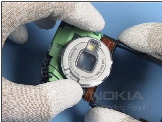
8. Align it and push down the assembly as shown evenly to fix the adhesive.
