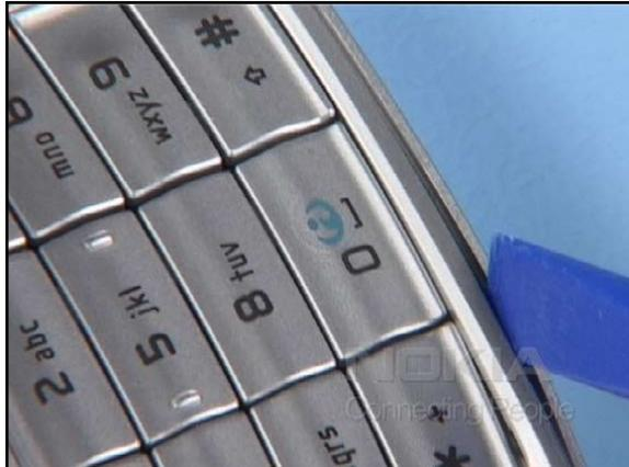
8. Gently pry open both plastic clips of the ITU KEYPAD.
