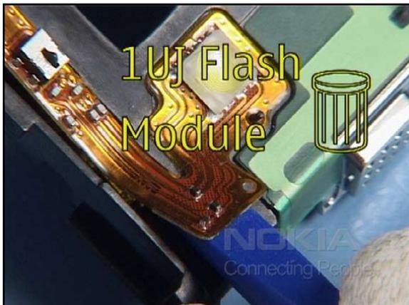
34. Now release the still fixed side with the SS-93. The module can't be used again.
