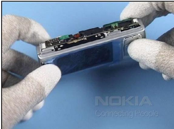
10. Shift the assembly together and turn it to access the screws.
