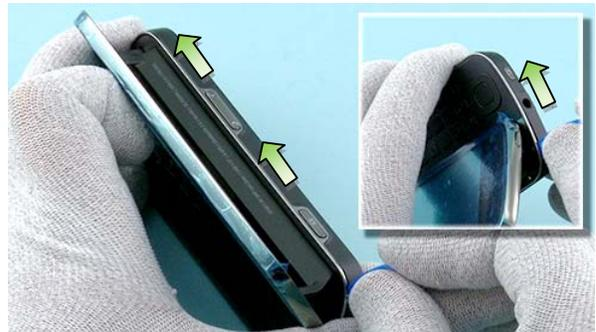
10) Slide the SRT-6 along the cover to release all the clips.
