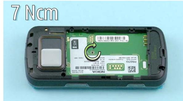
2) Tighten the TORX + size 4 screw to the torque of 7 Ncm.
