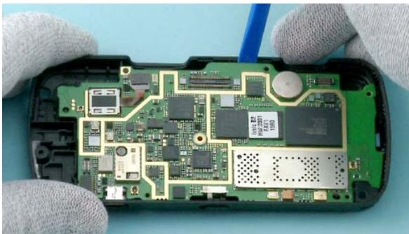
21) Release the engine board with the SS-93.
