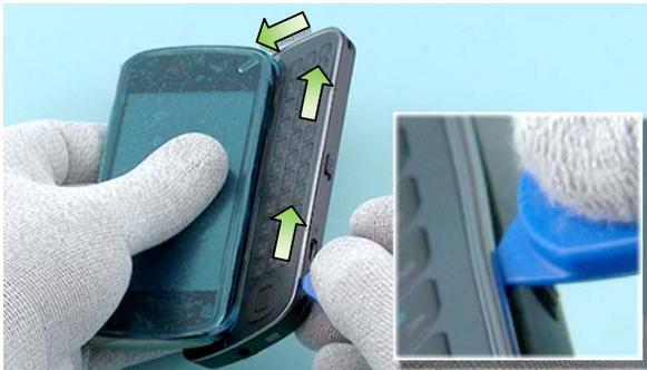
9) Open the slide and use the SRT-6 to release the clips of the lower part.
