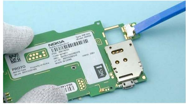
26) Release the HEAT SINK ASSEMBLY with the SS-93 and then remove the assembly.
