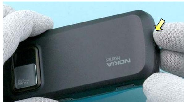
4) Press release button and remove the BATTERY COVER.
