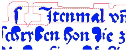
Fig. 31: Combining chosen contours to a new layout element.
