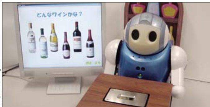
The infrared sommelier uses spectroscopic analysis to taste red or white wine.
