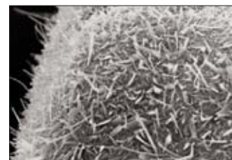
The starting point is a 20–40 \mu\text{m} thick film synthesized from a family of compounds known as diarylethenes (left). When the researchers shine UV light on the surface, small fibres approximately 1 \mu\text{m} in diameter begin to grow. This creates a super-water-repellent surface exhibiting the same properties as the lotus blossom (right).
