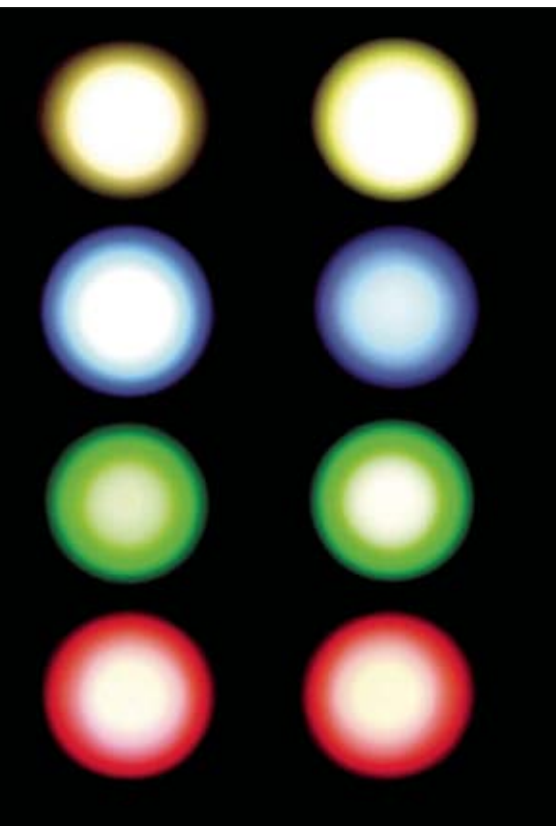
emitting in the white, red, blue and green, by attaching phosphors lead to phosphor-free ZnO LEDs serving all these colours.
