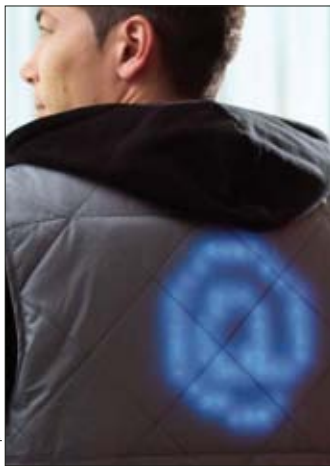
Lumalive jackets contain panels up to 200 × 200 mm 2 that can display logos and messages. Philips Research says that it is now ready to be commercialized.
