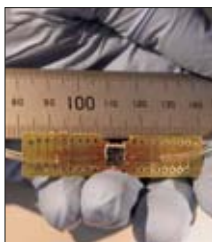
Chip combines microfluidics and integrated optics. p23
