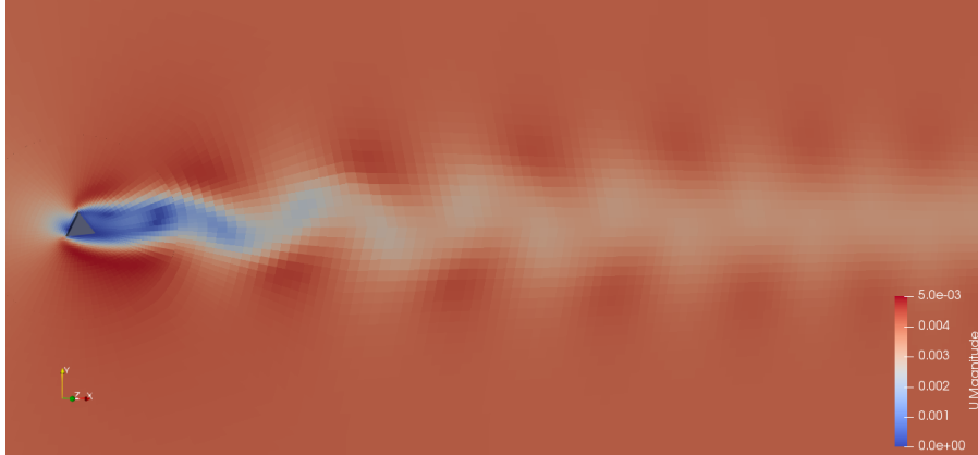
Figure 61: A 2D simulation of the triangular, prismatic body in laminar cross-flow using AMI to connect the body fitted mesh of the inner region with the mesh of the outer domain.
