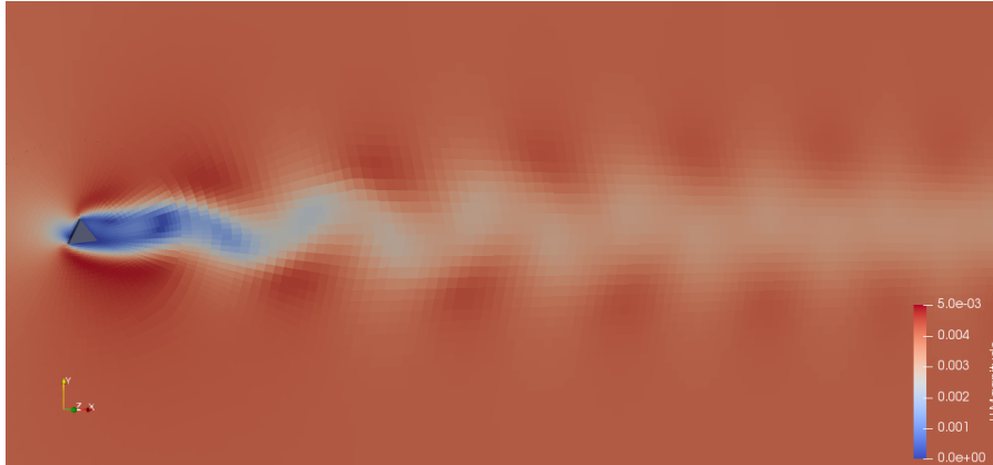
Figure 53: A 2D simulation of the triangular, prismatic body in laminar cross-flow using AMI to connect the body fitted mesh of the inner region with the mesh of the outer domain.
