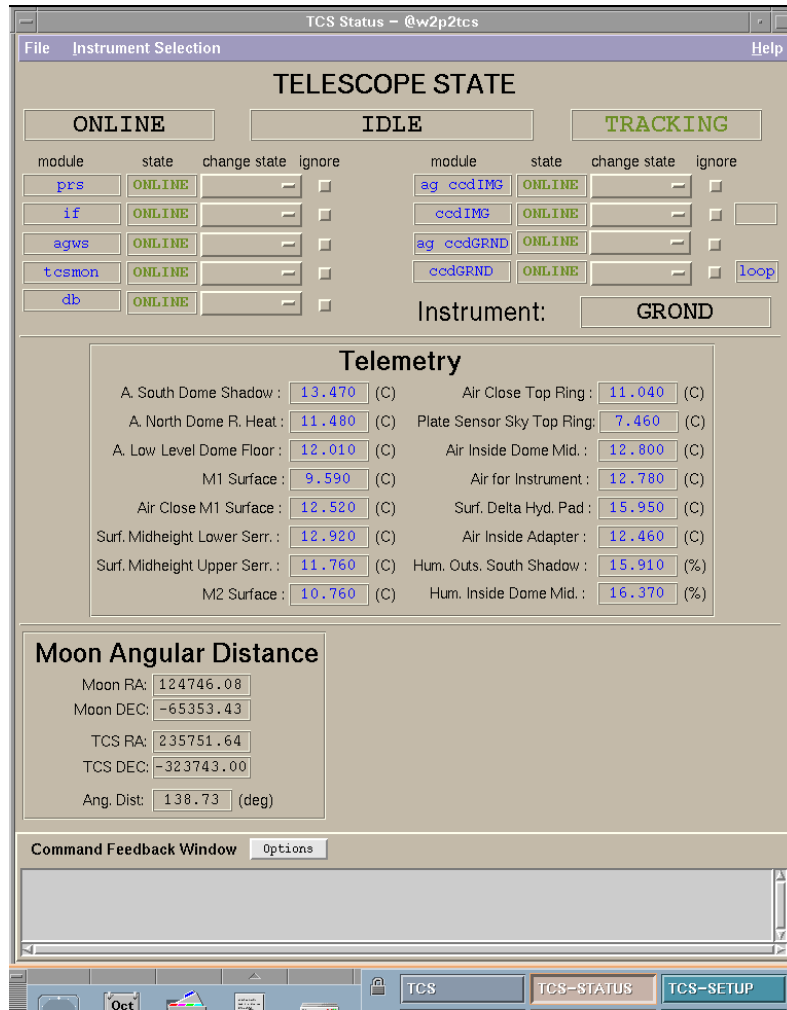
Figure 10.4: The TCS status window is mostly used to switch the pointing model between instruments.
