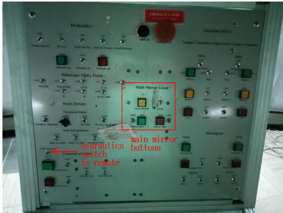
Figure 9.8: Controlling the hydraulics and mirror cover.
