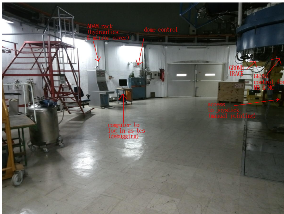
Figure 1.5: Entering the dome, from left to right: the ADAM controls, a computer to use the TCS , the dome controls, the bottom of the telescope.
