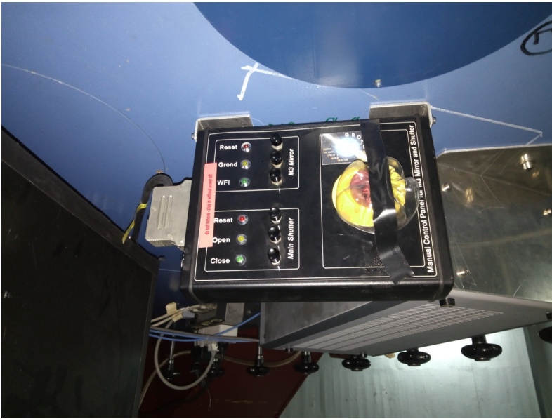
Figure 9.11: The GROND mirror and main cover control box.
