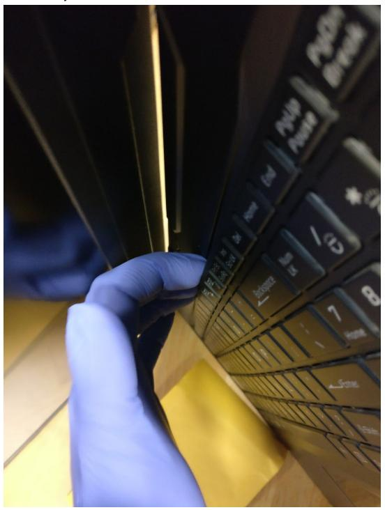
4. Flip over the keyboard and remove the 4 silver screws and 1 black screw. Their location is highlighted in red. (Note: In this photo, the screws have already been removed.)
