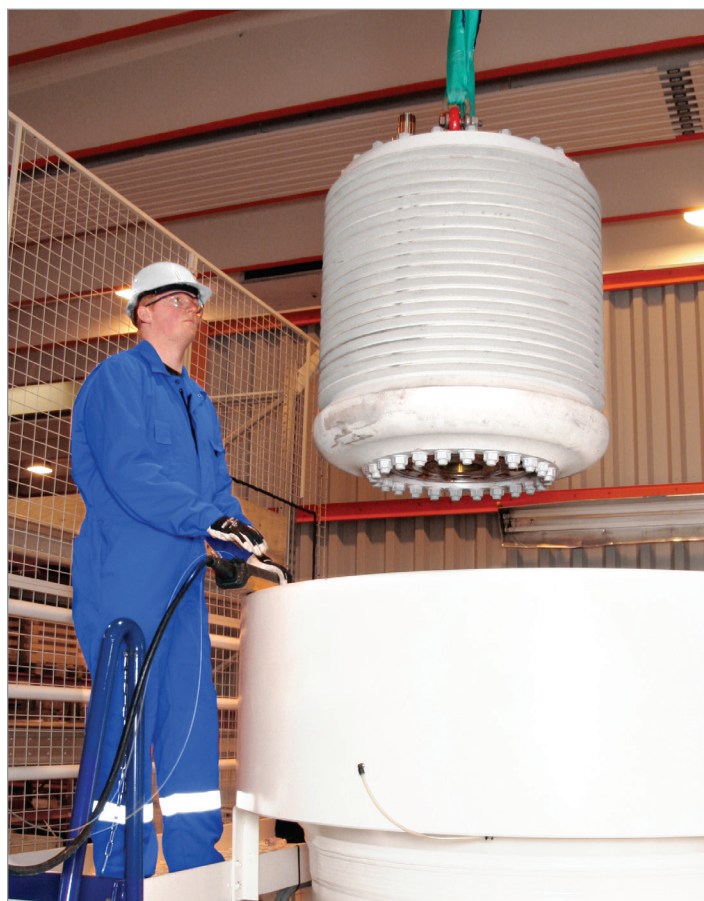
At the OneSubsea facility in Horsøy, Norway, PhaseWatcher flowmeters undergo rigorous testing at pressures exceeding the expected pressure on the seabed.
